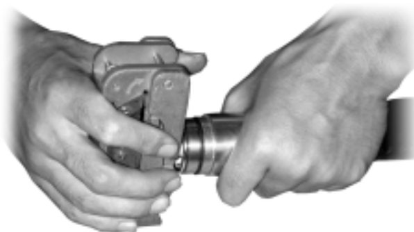
Fig. 8.6-5 Schematic Diagram of Expanding the External Copper Conductor
