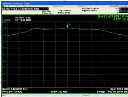
In-Band Reference Level BLE 1M_Channel 39
