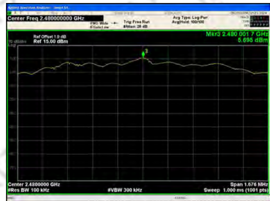
In-Band Reference Level BLE 2M_Channel 39
