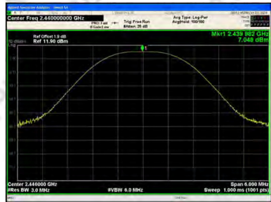
Peak Output Power BLE 1M_Channel 19
