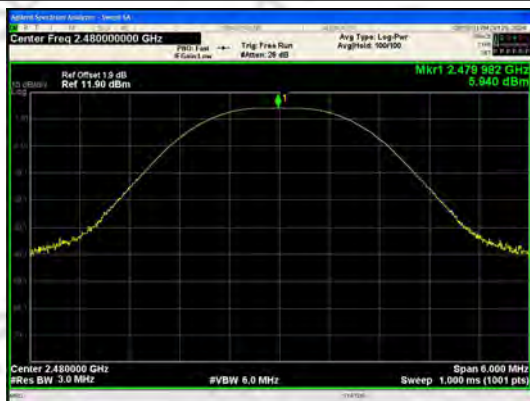
Peak Output Power BLE 1M_Channel 39
