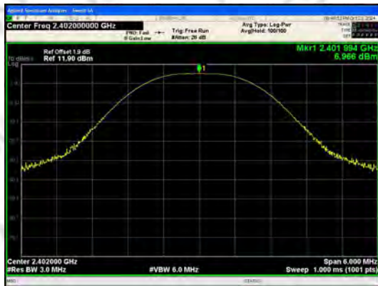
Peak Output Power BLE 1M_Channel 0
