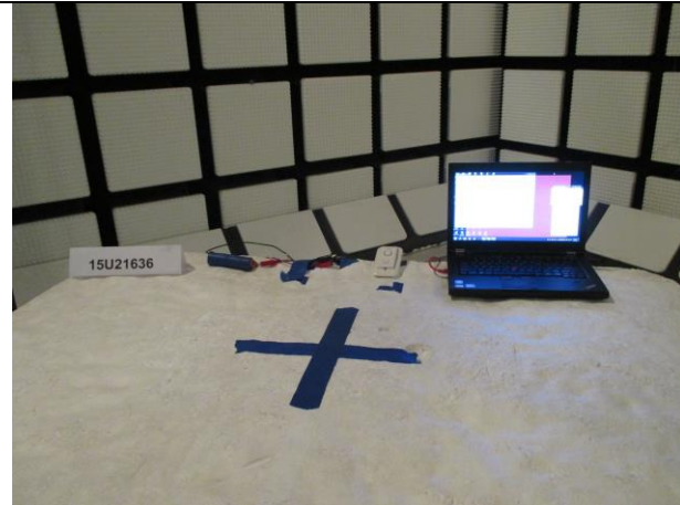
RADIATED FRONT PHOTO (BELOW 1 GHz)
