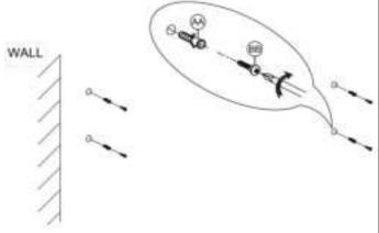
**4B.4)** With the help of another person, lift the fire box(A) and hang up the fire box onto the wall with the screw(BB).
