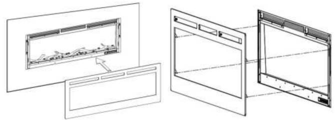
**4.A10)** Fix the glass front by screws (CC) and complete the installation.
