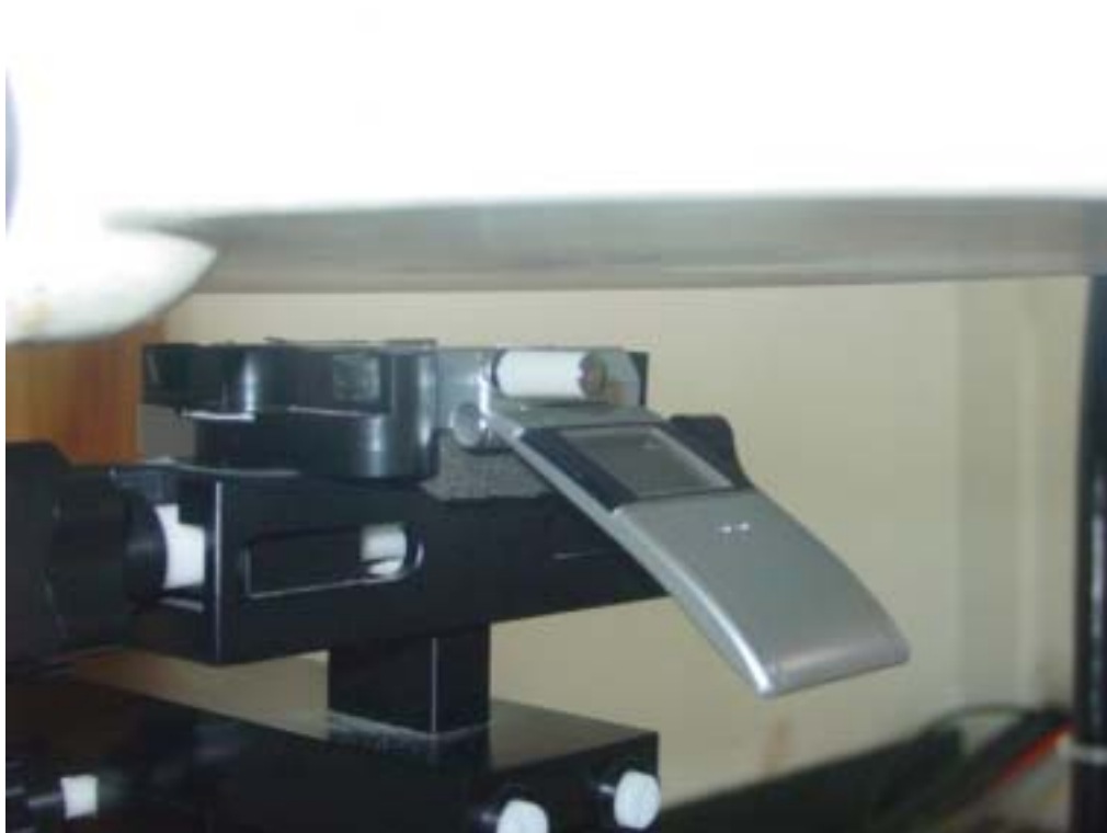
Picture 6 Flat Phantom -- Body-worn Position (toward ground, the distance from handset to the bottom of the Phantom is 1.5cm)
