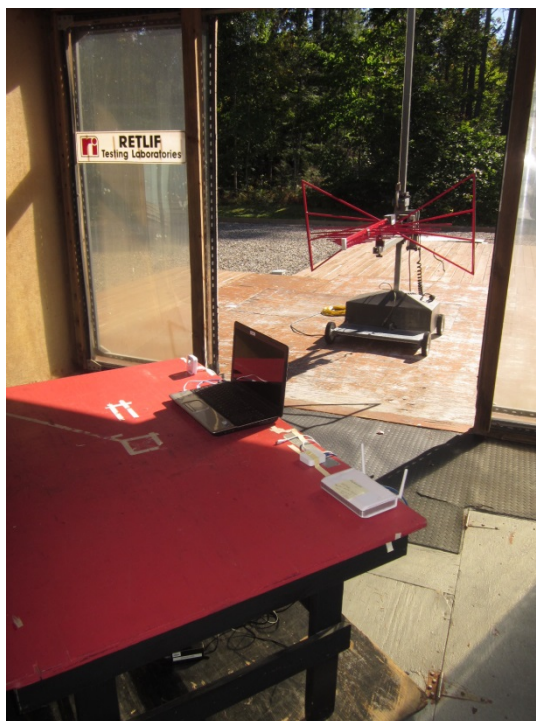
Horizontal Antenna Polarization, 25 MHz – 1 GHz
