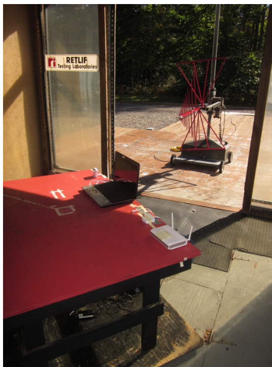
Vertical Antenna Polarization, 25 MHz – 1 GHz
