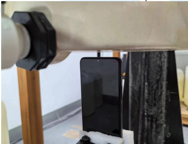
Top Side of EUT with 1 cm Gap
