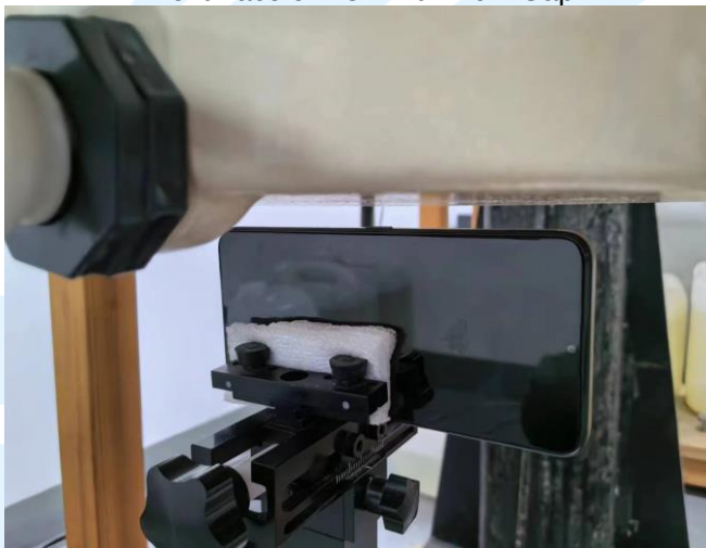
Left Side of EUT with 1 cm Gap
