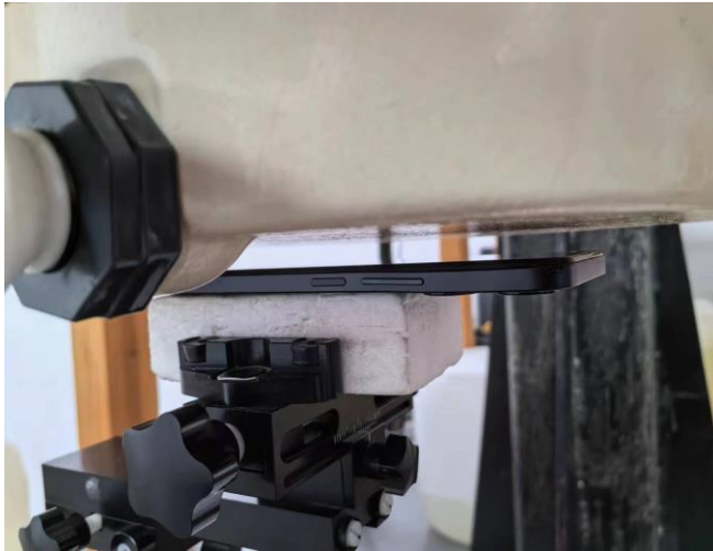
Front Face of EUT with 1 cm Gap
