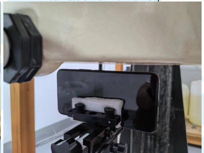
Right Side of EUT with 1 cm Gap
