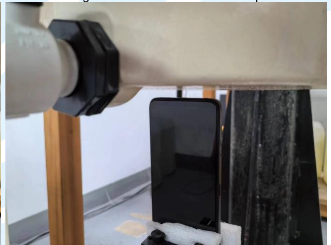
Bottom Side of EUT with 1 cm Gap
