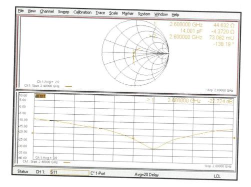
Impedance Measurement Plot for Body TSL
