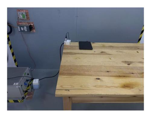
Set-up for Radiated Emission (RE), Below 1GHz
