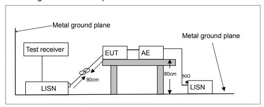
LISN: Line Impedance Stabilization Network
