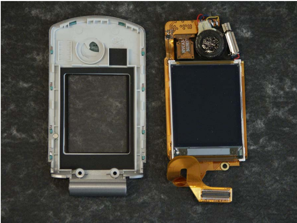
Photo 4. Internal Display and Flexible PCB (left)
