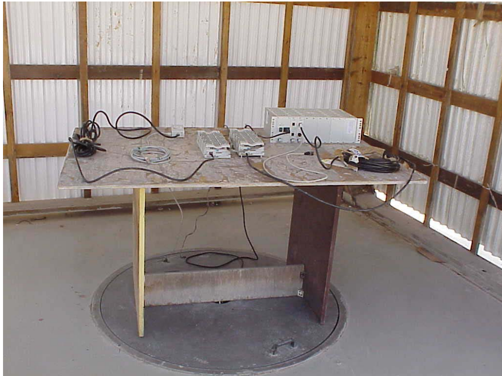
Photo # 3. Base Station + Subscriber Unit Radiated emission test on open site
