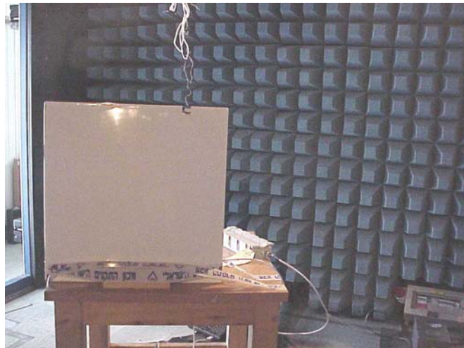
Photo # 7. Radio unit with Unidirectional antenna UNI-28-4 P/N AN1230 Spurious emission test
