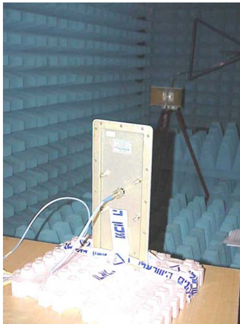
Photo # 5. P/N AN1152 Spurious emission test
