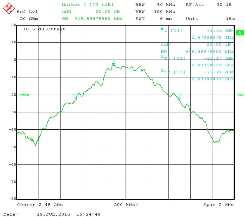
**EDR ( $\pi/4$ -DQPSK): Low Channel**
