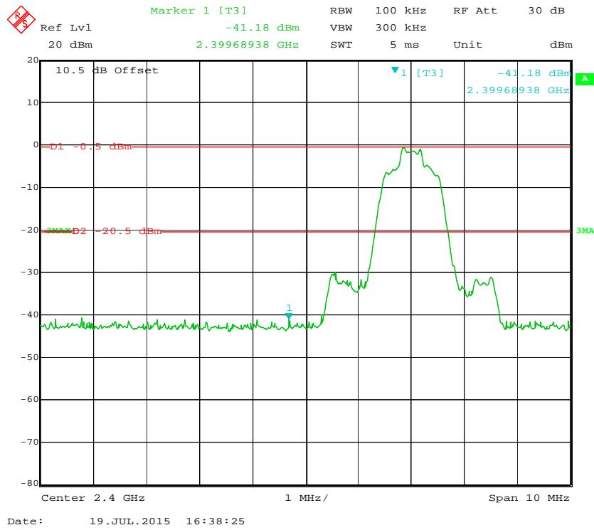
**EDR ( $\pi/4$ -DQPSK): Band Edge-Right Side**
