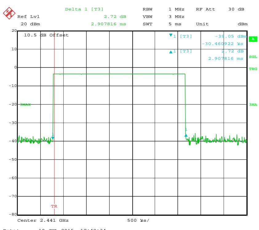
**Pulse time, High Channel, DH5**
