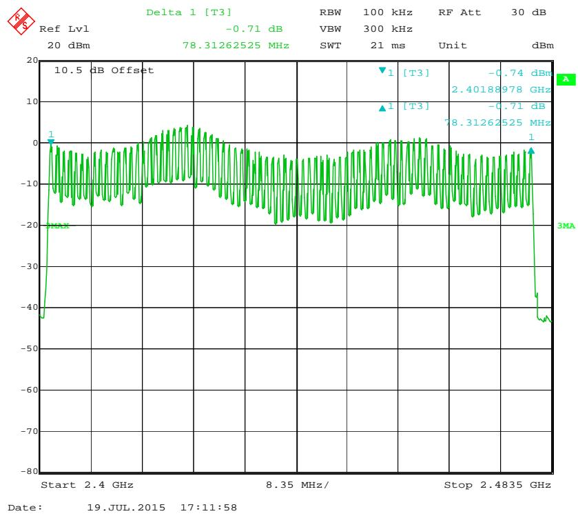
**EDR ( $\pi/4$ -DQPSK): Number of Hopping Channels**
