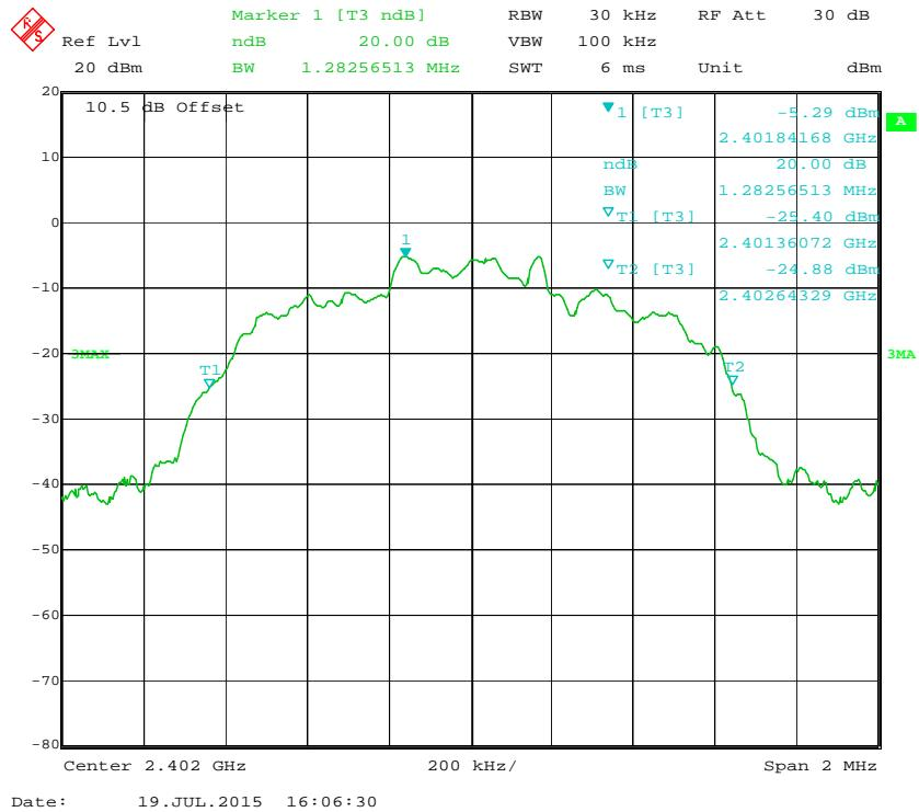
**EDR (8DPSK): Middle Channel**
