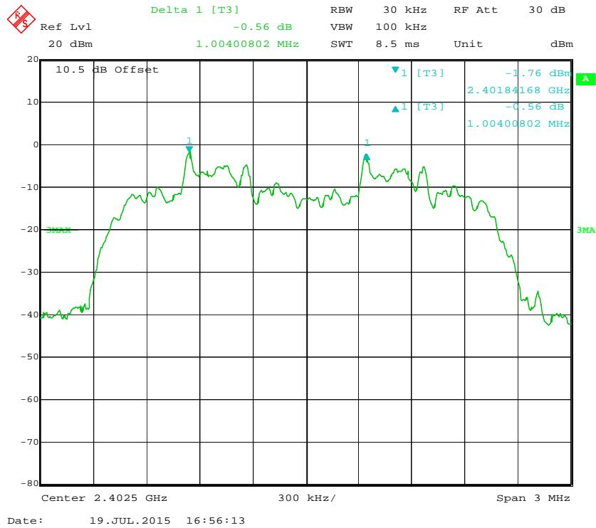
**EDR ( $\pi/4$ -DQPSK): Middle Channel**
