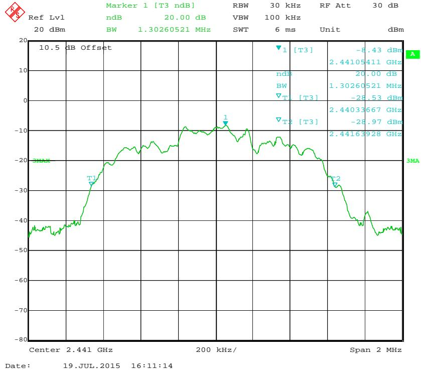
**EDR ( $\pi/4$ -DQPSK): High Channel**
