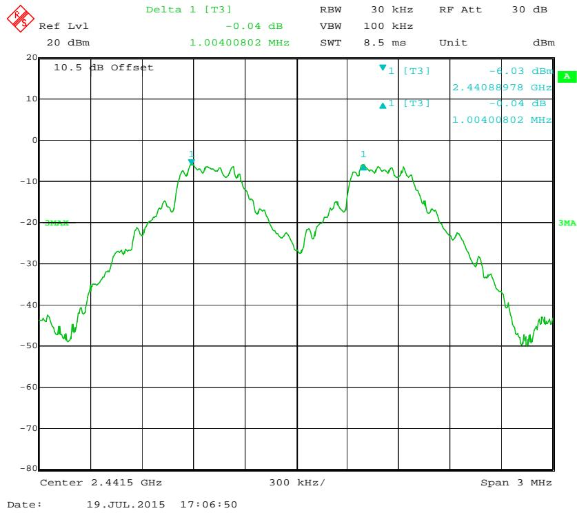
**BDR (GFSK): High Channel**
