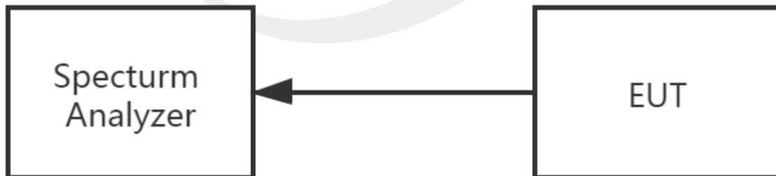
The EUT is connected to the Spectrum Analyzer; the RF load attached to the EUT antenna terminals is 50 Ohm; the path loss as the factor is calibrated to correct the reading. Make the measurement with the spectrum analyzer's resolution bandwidth(RBW) = 100 kHz. In order to make an accurate measurement, set the span greater than RBW.
