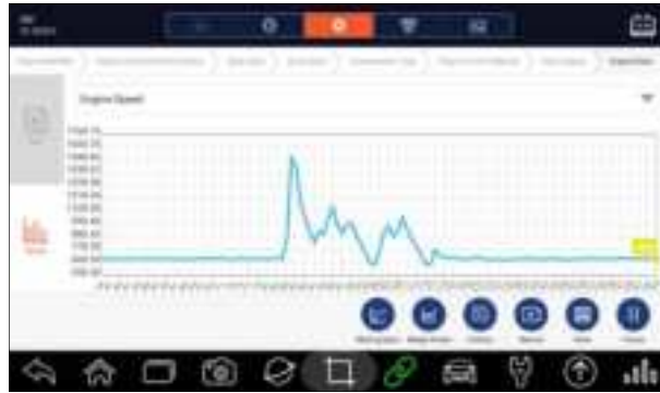
Figure 5-20 Sample PID Graph Screen
