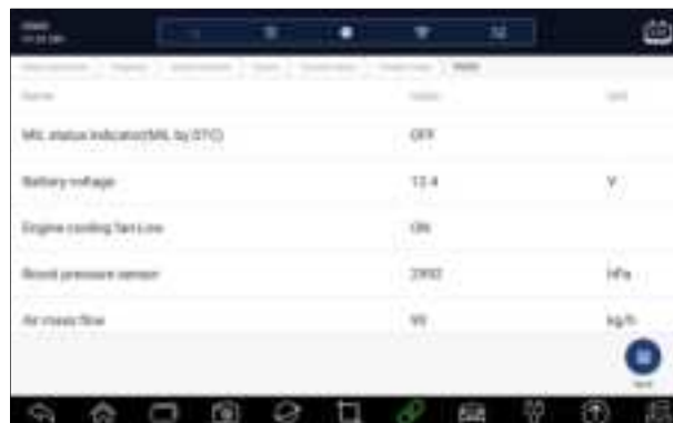
Figure 5-13 Sample Freeze Frame Screen
