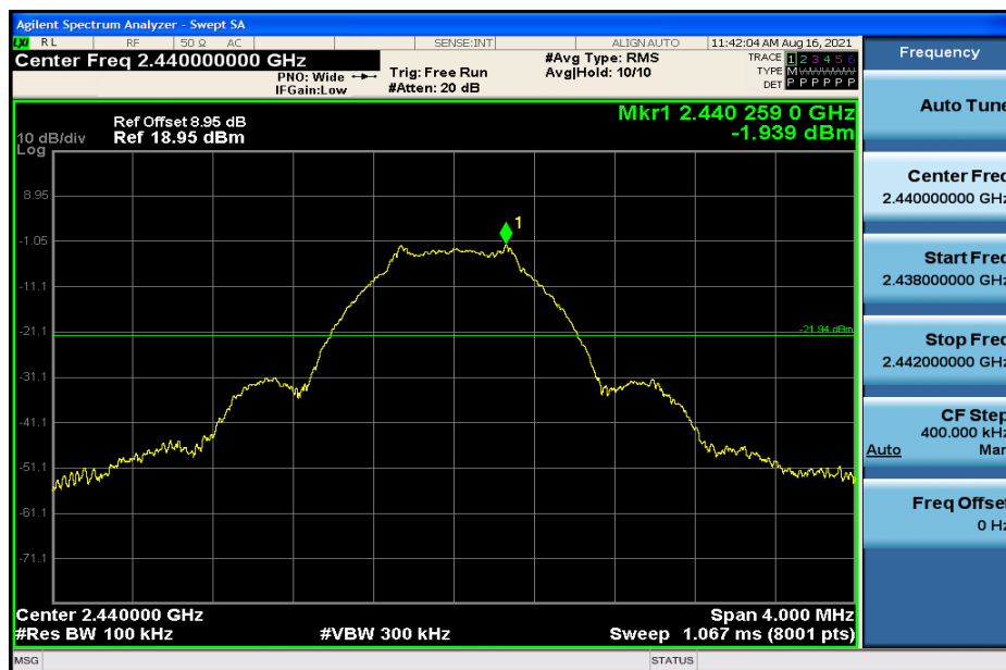
RF Conducted Spurious Emissions_BLE_2440
