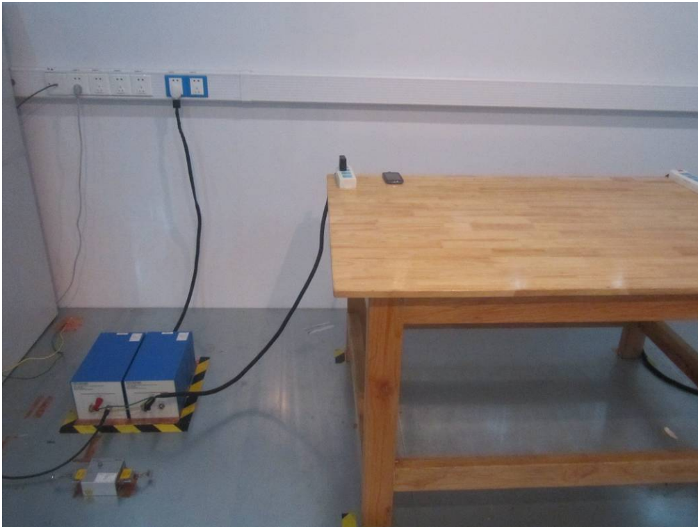
Conducted Emissions Test Setup Front View
