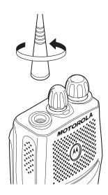
Turn the antenna counter-clockwise to remove it.
