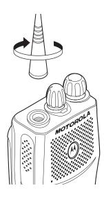
Turn the antenna clockwise to attach it.
