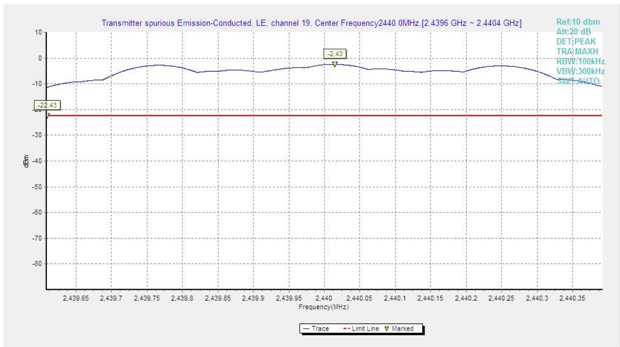
Fig.12 Conducted Spurious Emission (Ch19, Center Frequency)
