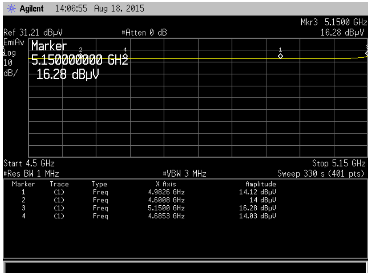
Figure 61. Restricted Band 4.5 - 5.15 GHz operating on Channel 36, 802.11n - Average on Chip Antenna
