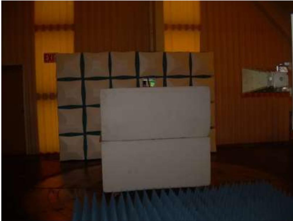
**Photograph 3: Front View Radiated Emissions Configuration – Above 1000 MHz – C4-T4IW10 Shown**
