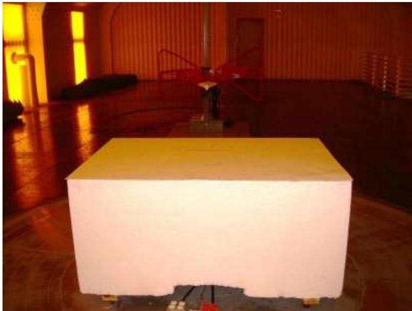
**Photograph 13: Reference Photo of Test Setup for Emissions From 30 MHz to 1000 MHz**
