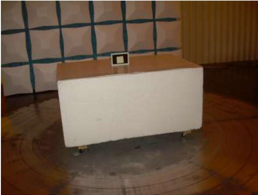
**Photograph 1: Front View Radiated Emissions Configuration – Below 30 MHz – C4-T4IW10 Shown**
