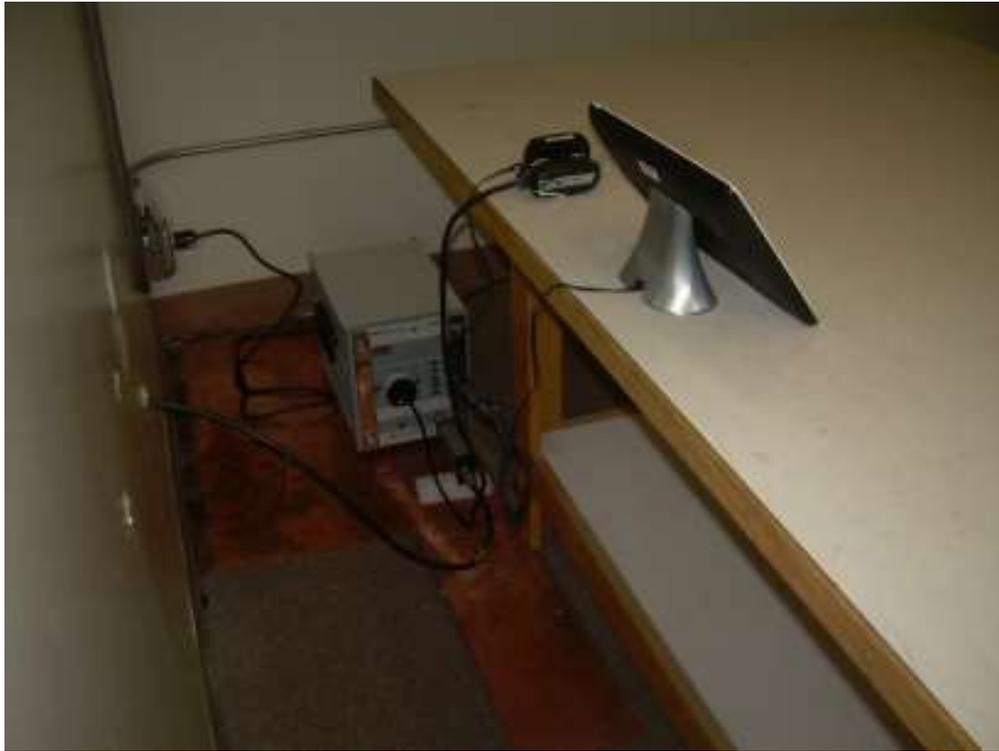
**Photograph 9: Back View Conducted Emissions Worst-Case Configuration T4T10 Shown**
