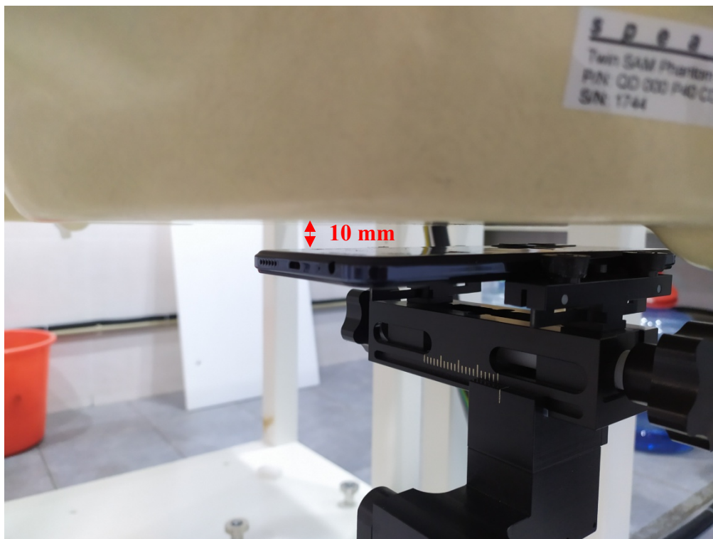
Body (Worn) Back Setup Photo (10mm)
