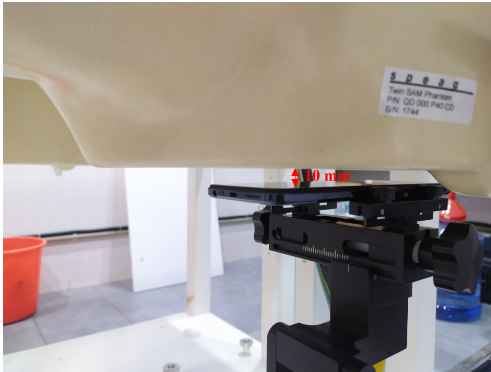
Body Front Setup Photo (10mm)
