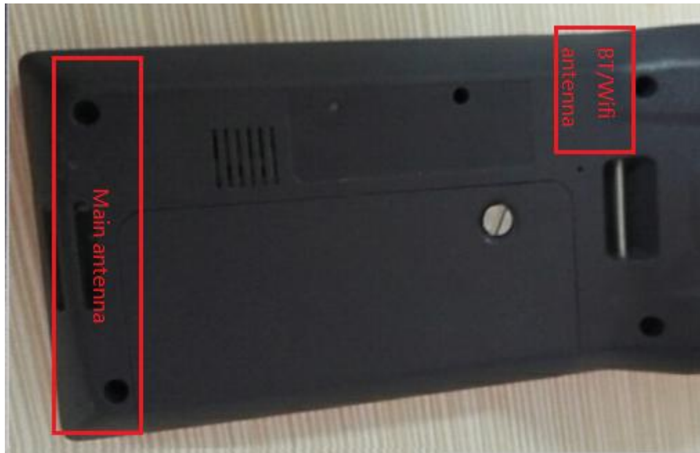
Picture of antennas
