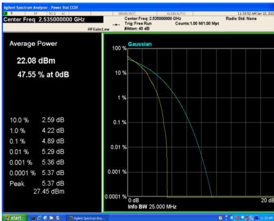
Band7 QPSK BW=20MHz Channel=21100 RB Size=1 Position=#0
