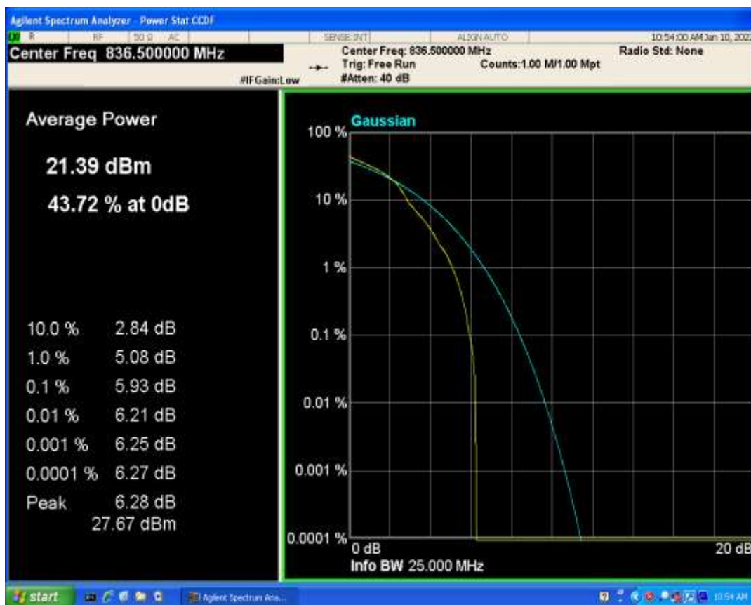
Band5 QAM16 BW=1.4MHz Channel=20525 RB Size=1 Position=#0
