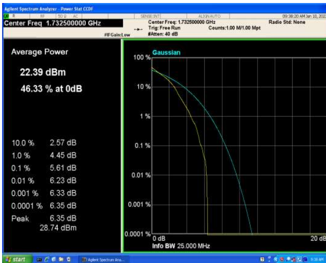
Band4 QAM16 BW=5MHz Channel=20175 RB Size=1 Position=#0
