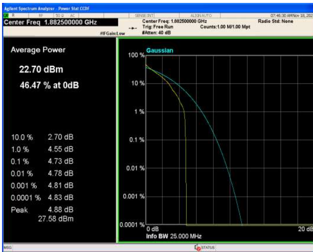
Band25 QPSK BW=5MHz Channel=26365 RB Size=1 Position=#0
