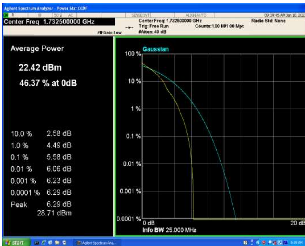
Band4 QPSK BW=20MHz Channel=20175 RB Size=1 Position=#0
