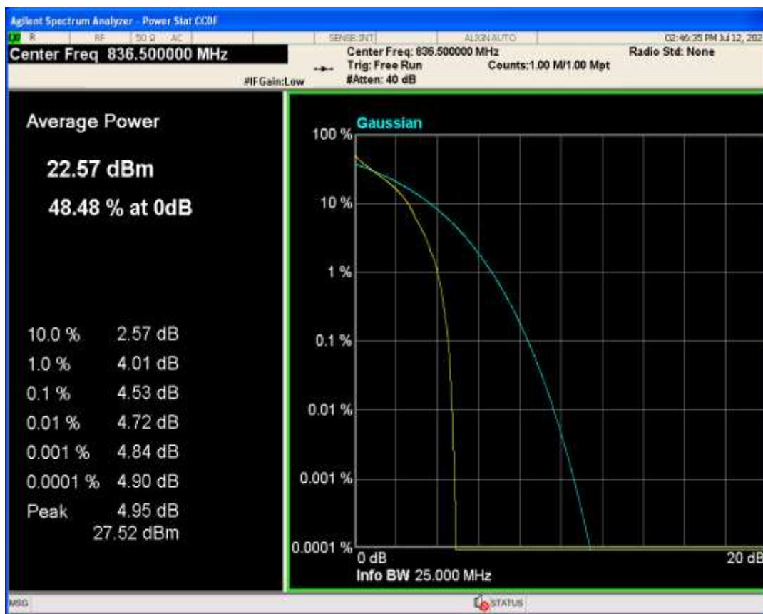
Band26b QPSK BW=5MHz Channel=26915 RB Size=1 Position=#0
