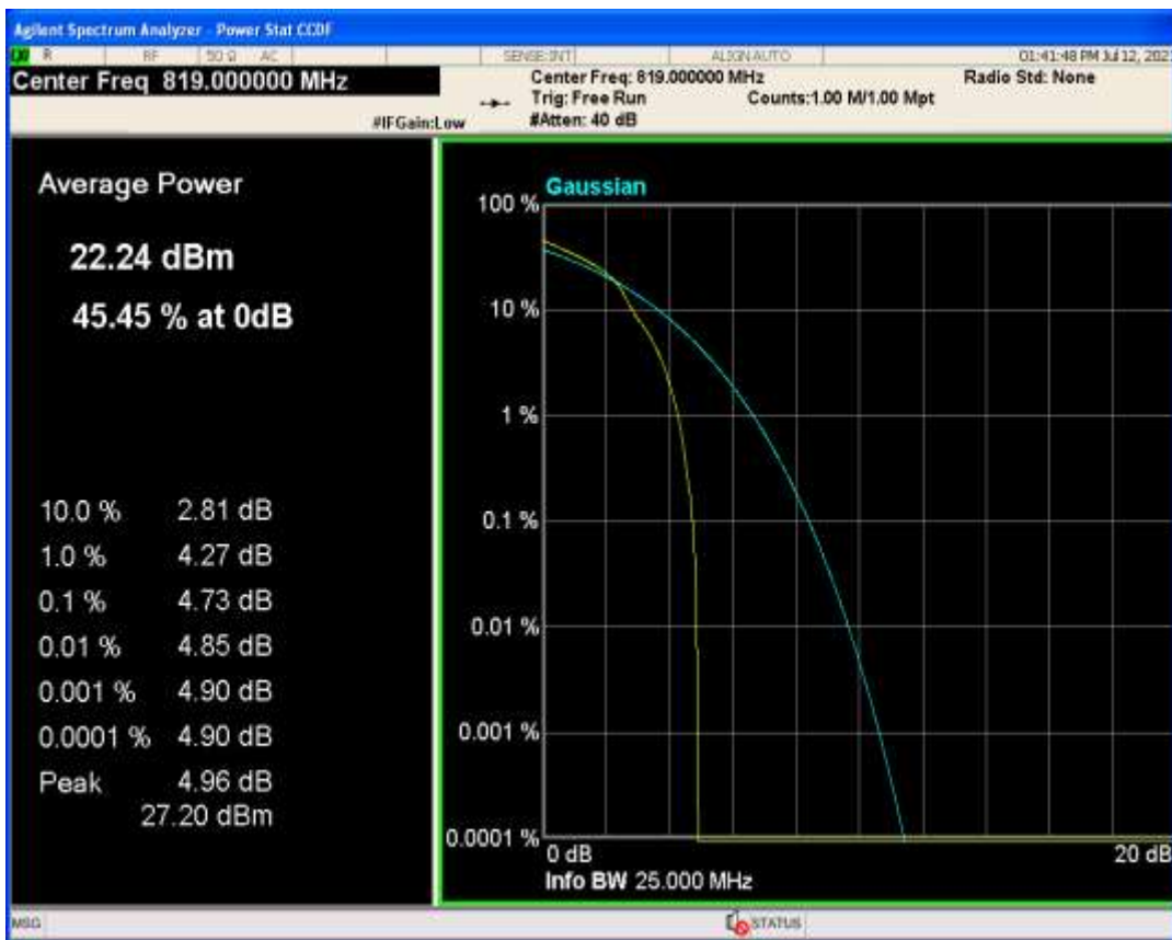
Band26a QPSK BW=1.4MHz Channel=26740 RB Size=1 Position=#0
