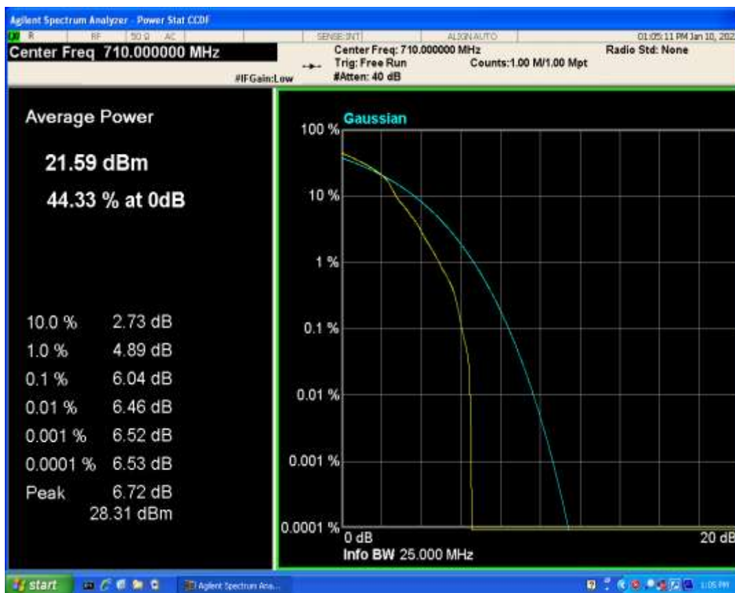
Band2 QAM16 BW=1.4MHz Channel=18900 RB Size=1 Position=#0
