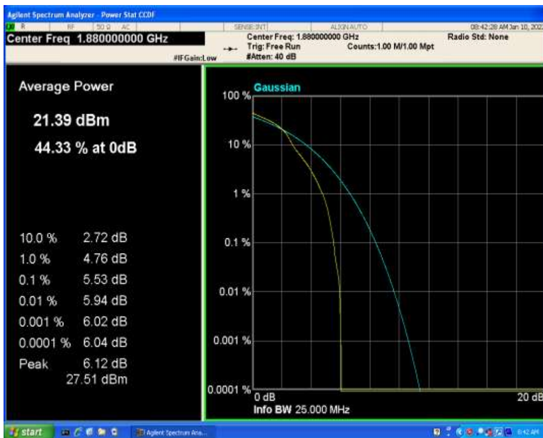
Band2 QAM16 BW=20MHz Channel=18900 RB Size=1 Position=#0
