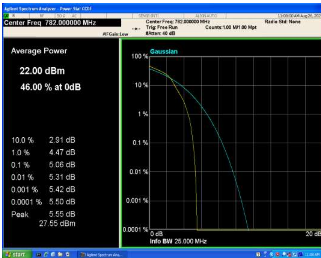
Band13 QAM16 BW=5MHz Channel=23230 RB Size=1 Position=#0
