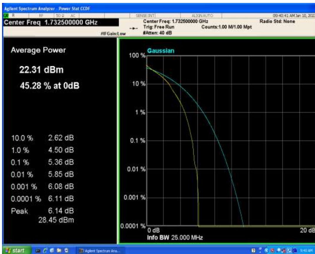
Band5 QAM16 BW=10MHz Channel=20525 RB Size=1 Position=#0
