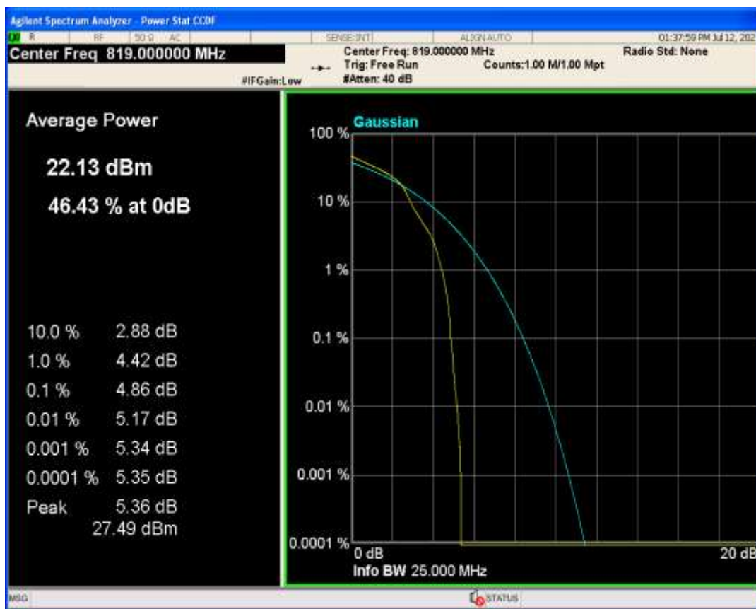
Band26a QAM16 BW=10MHz Channel=26740 RB Size=1 Position=#0
