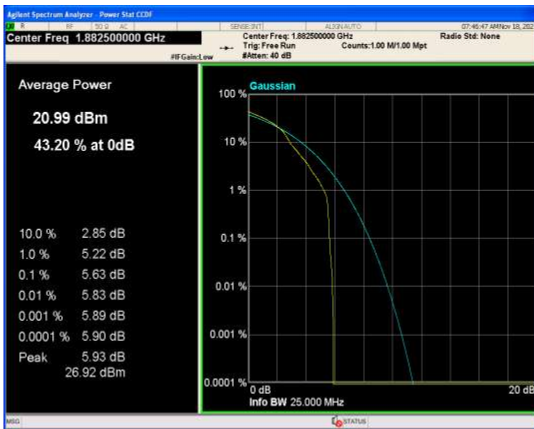
Band25 QAM16 BW=1.4MHz Channel=26365 RB Size=1 Position=#0
