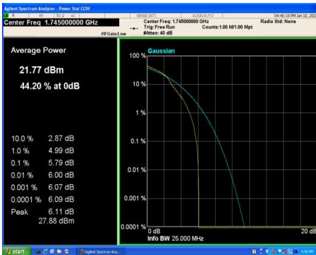
Band66 QPSK BW=15MHz Channel=132322 RB Size=1 Position=#0
