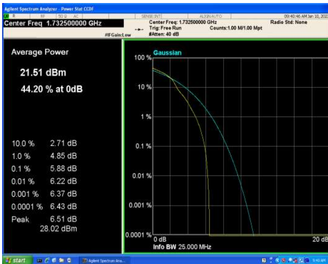
Band4 QPSK BW=5MHz Channel=20175 RB Size=1 Position=#0
