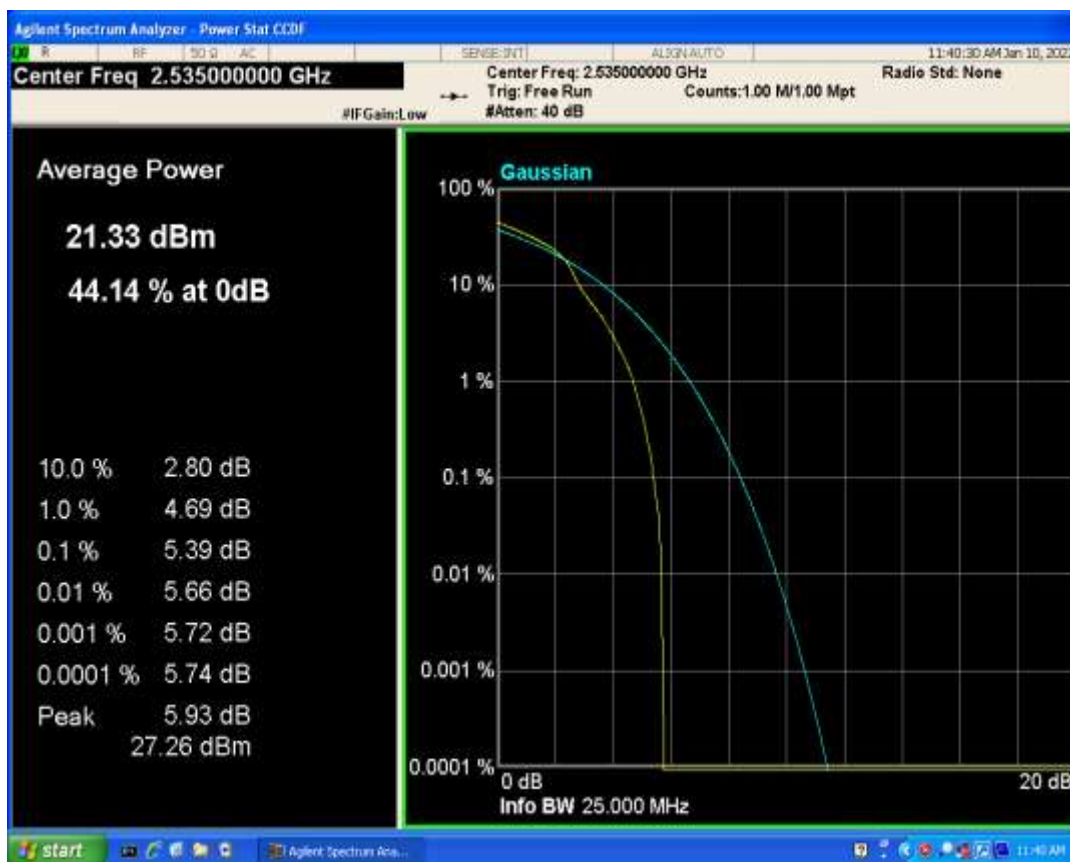
Band7 QAM16 BW=5MHz Channel=21100 RB Size=1 Position=#0
