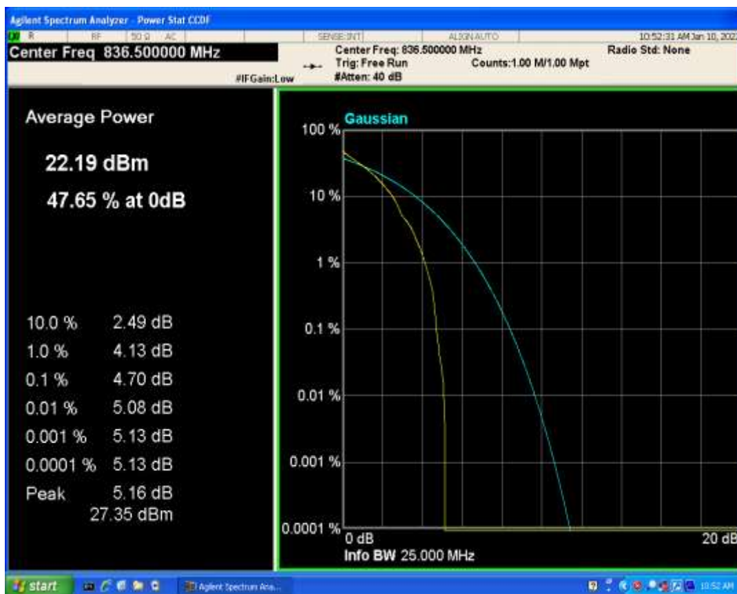
Band5 QPSK BW=5MHz Channel=20525 RB Size=1 Position=#0
