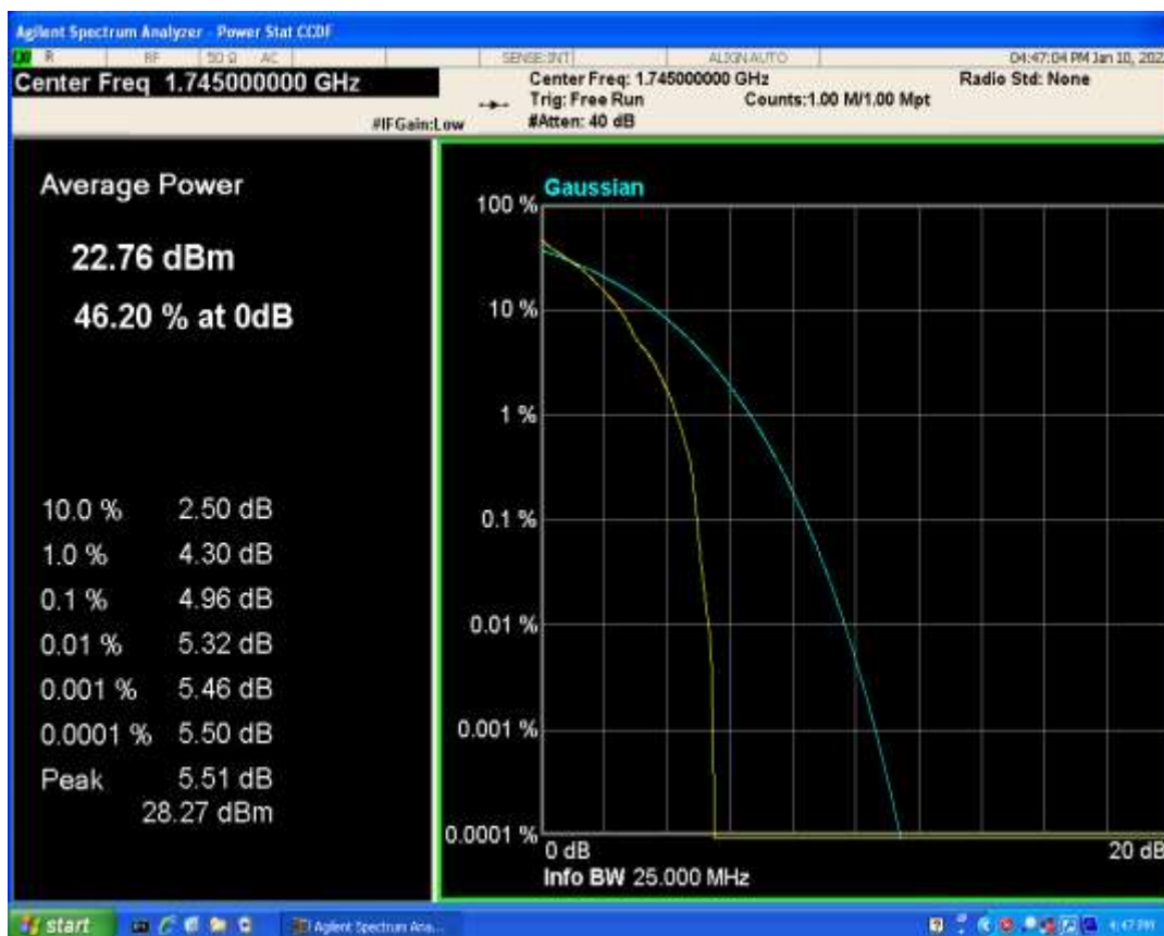
Band66 QPSK BW=20MHz Channel=132322 RB Size=1 Position=#0
