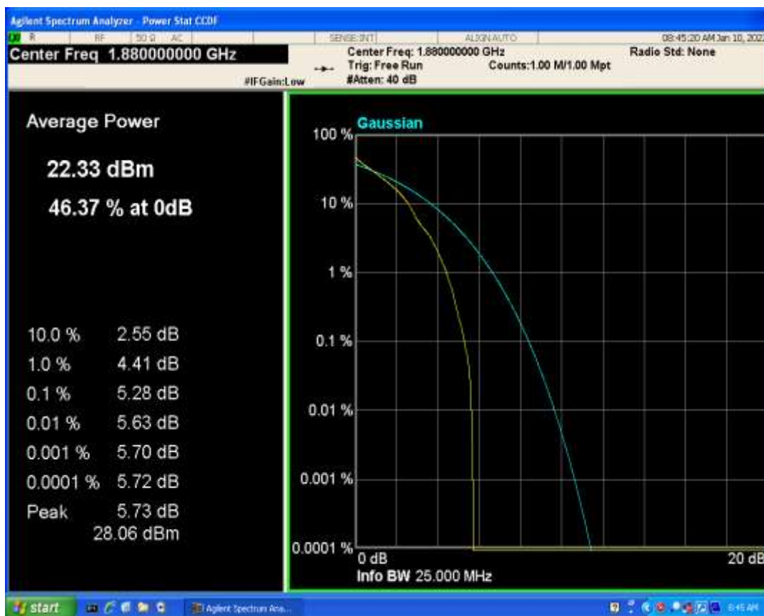
Band2 QAM16 BW=5MHz Channel=18900 RB Size=1 Position=#0
