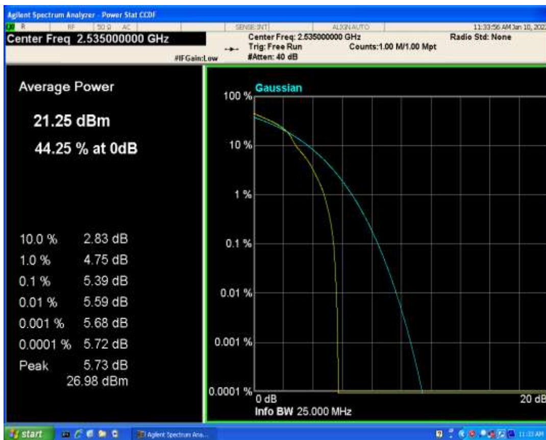
Band7 QPSK BW=10MHz Channel=21100 RB Size=1 Position=#0
