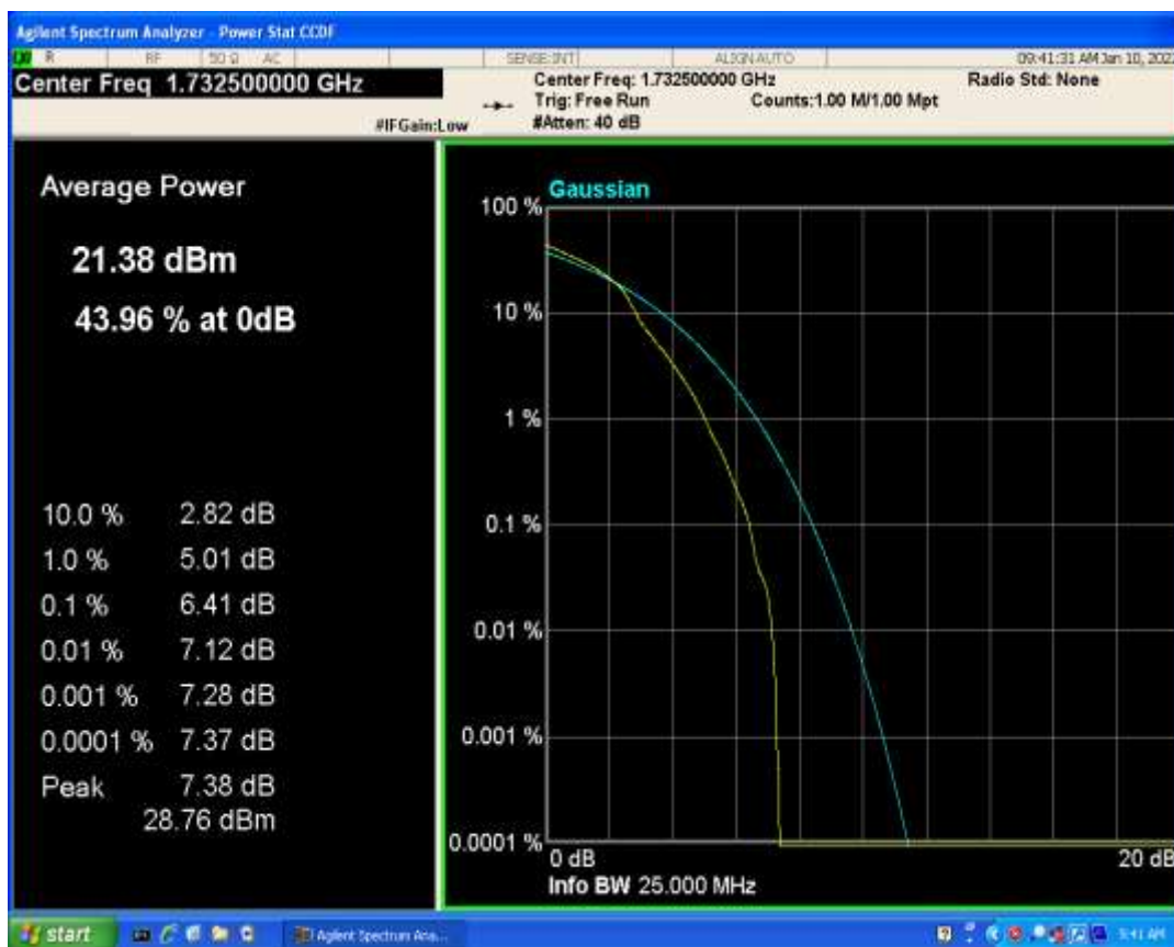
Band4 QAM16 BW=1.4MHz Channel=20175 RB Size=1 Position=#0
