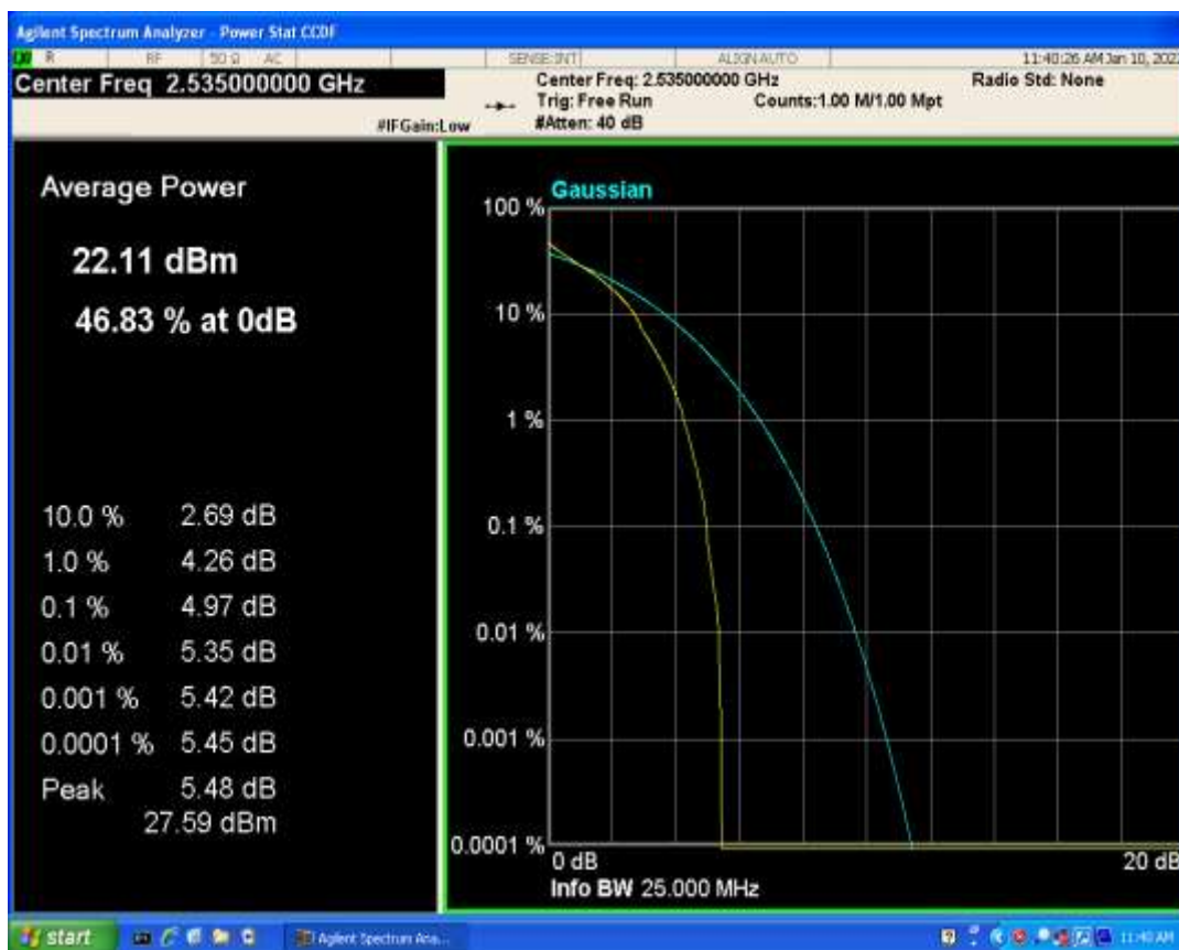
Band7 QPSK BW=15MHz Channel=21100 RB Size=1 Position=#0
