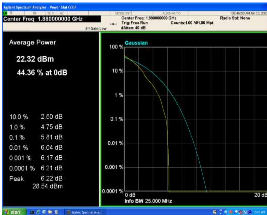
Band2 QPSK BW=10MHz Channel=18900 RB Size=1 Position=#0
