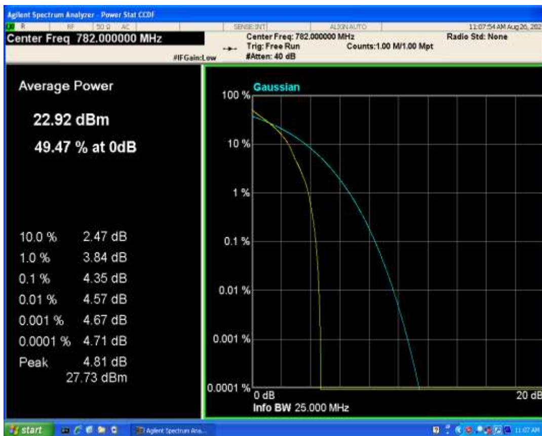
Band13 QPSK BW=5MHz Channel=23230 RB Size=1 Position=#0
