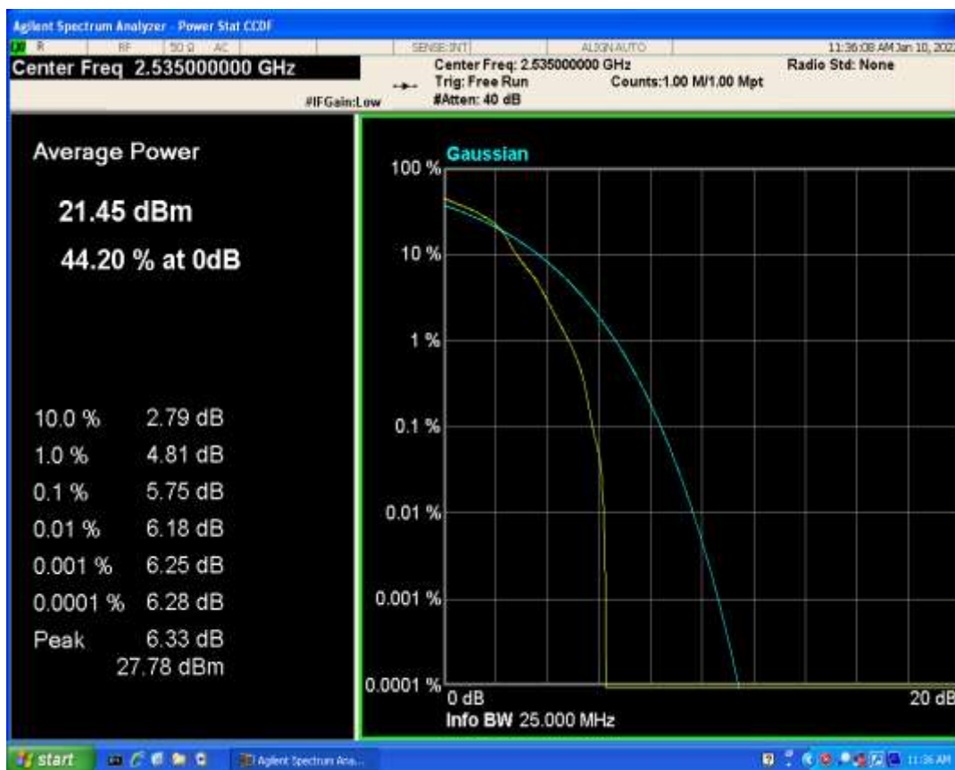
Band7 QAM16 BW=20MHz Channel=21100 RB Size=1 Position=#0
