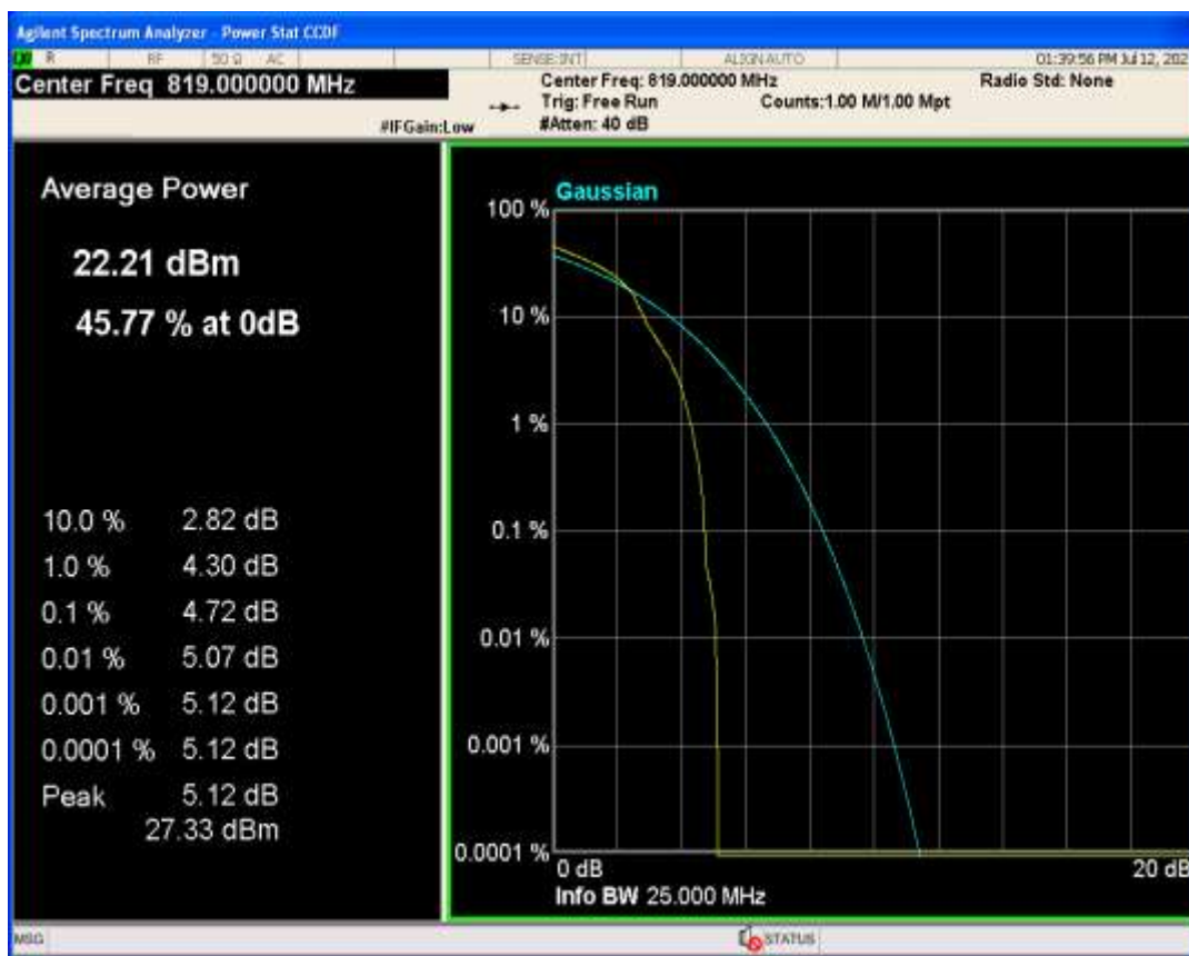
Band26a QAM16 BW=1.4MHz Channel=26740 RB Size=1 Position=#0
