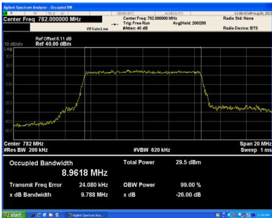
Band13 QPSK BW=5MHz Channel=23230 RB Size=25 Position=#0
