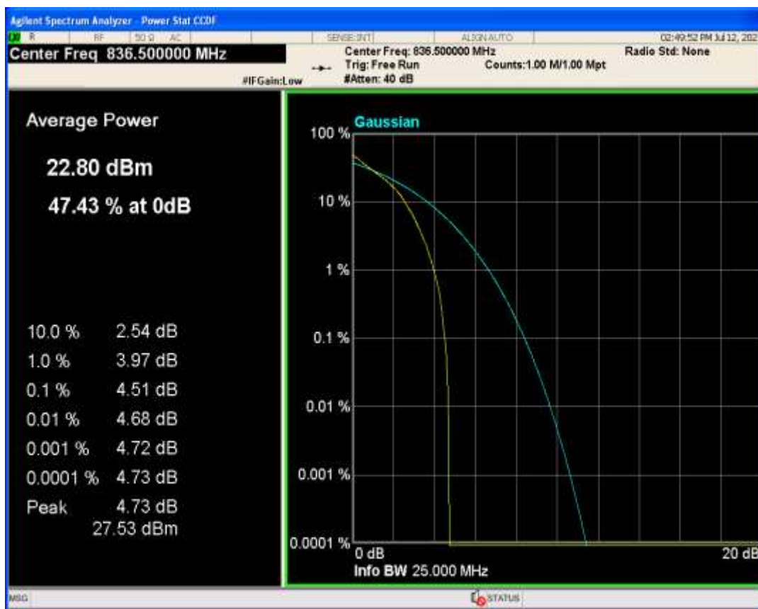
Band26b QPSK BW=3MHz Channel=26915 RB Size=1 Position=#0
