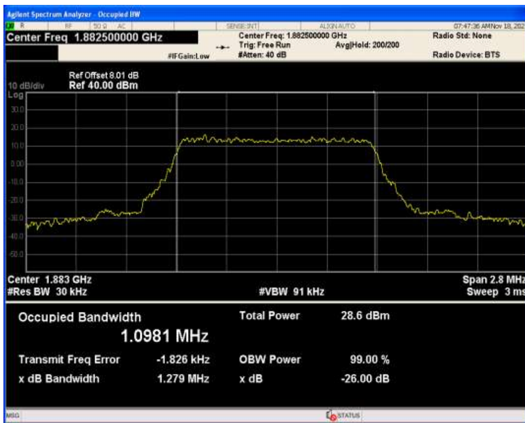
Band25 QAM16 BW=10MHz Channel=26365 RB Size=50 Position=#0
