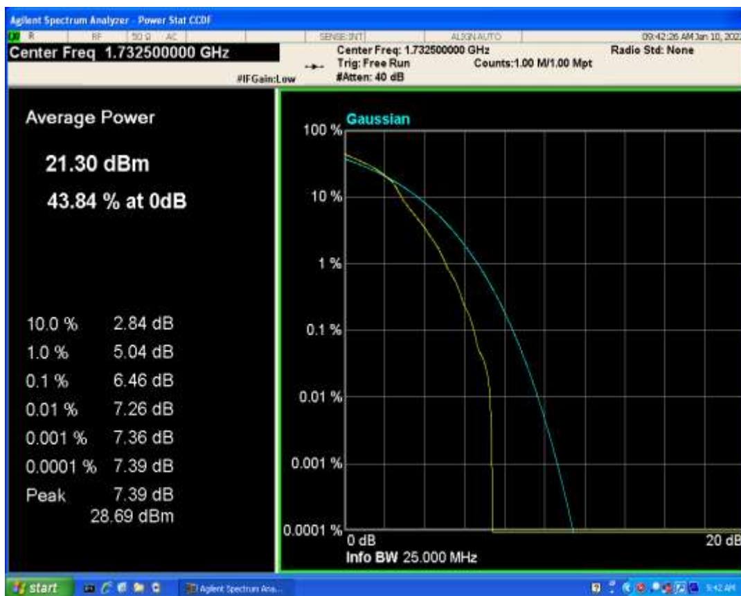
Band4 QAM16 BW=10MHz Channel=20175 RB Size=1 Position=#0
