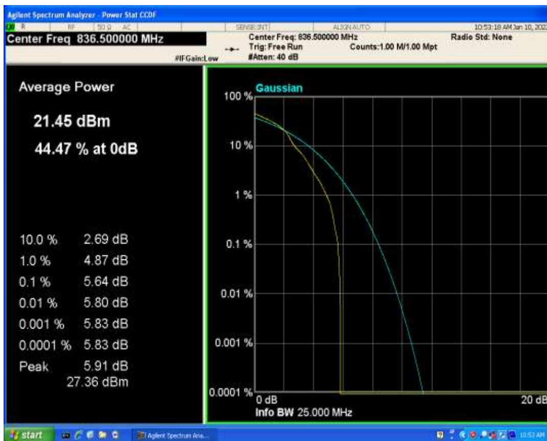
Band5 QPSK BW=1.4MHz Channel=20525 RB Size=1 Position=#0
