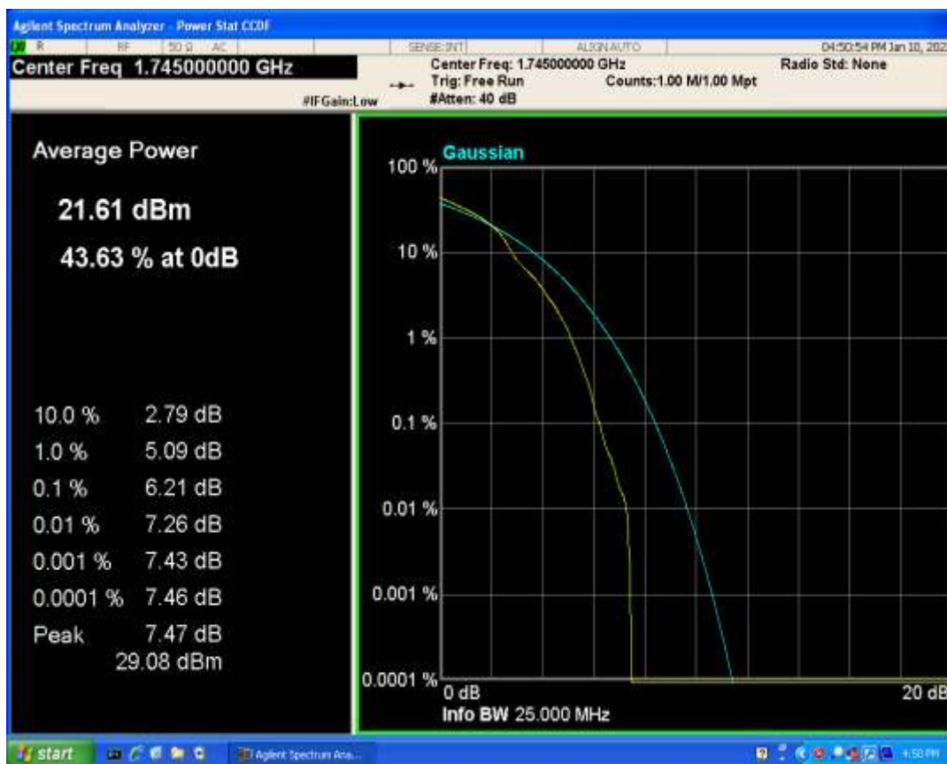
Band66 QAM16 BW=15MHz Channel=132322 RB Size=1 Position=#0
