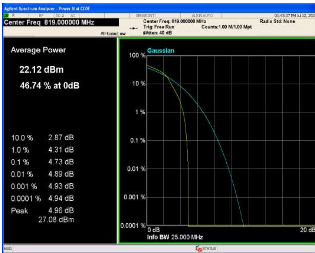
Band26a QPSK BW=5MHz Channel=26740 RB Size=1 Position=#0
