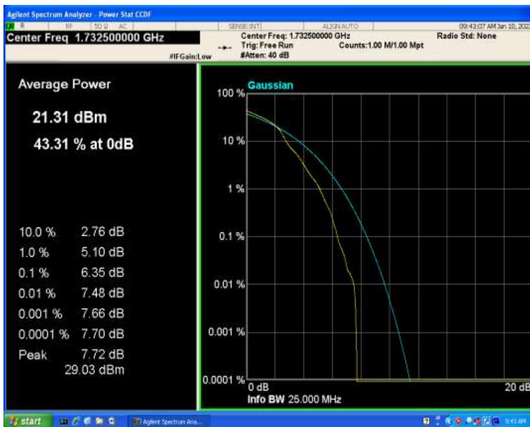
Band4 QPSK BW=1.4MHz Channel=20175 RB Size=1 Position=#0
