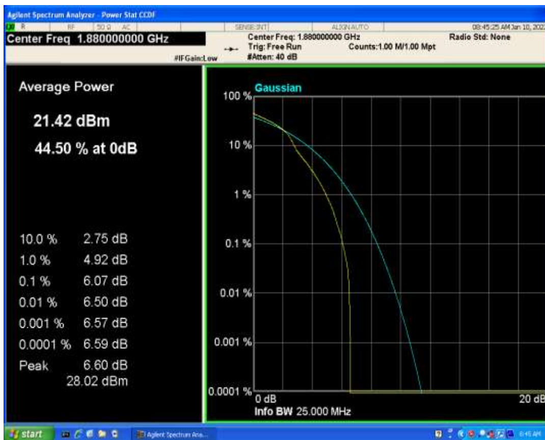
Band2 QAM16 BW=15MHz Channel=18900 RB Size=1 Position=#0
