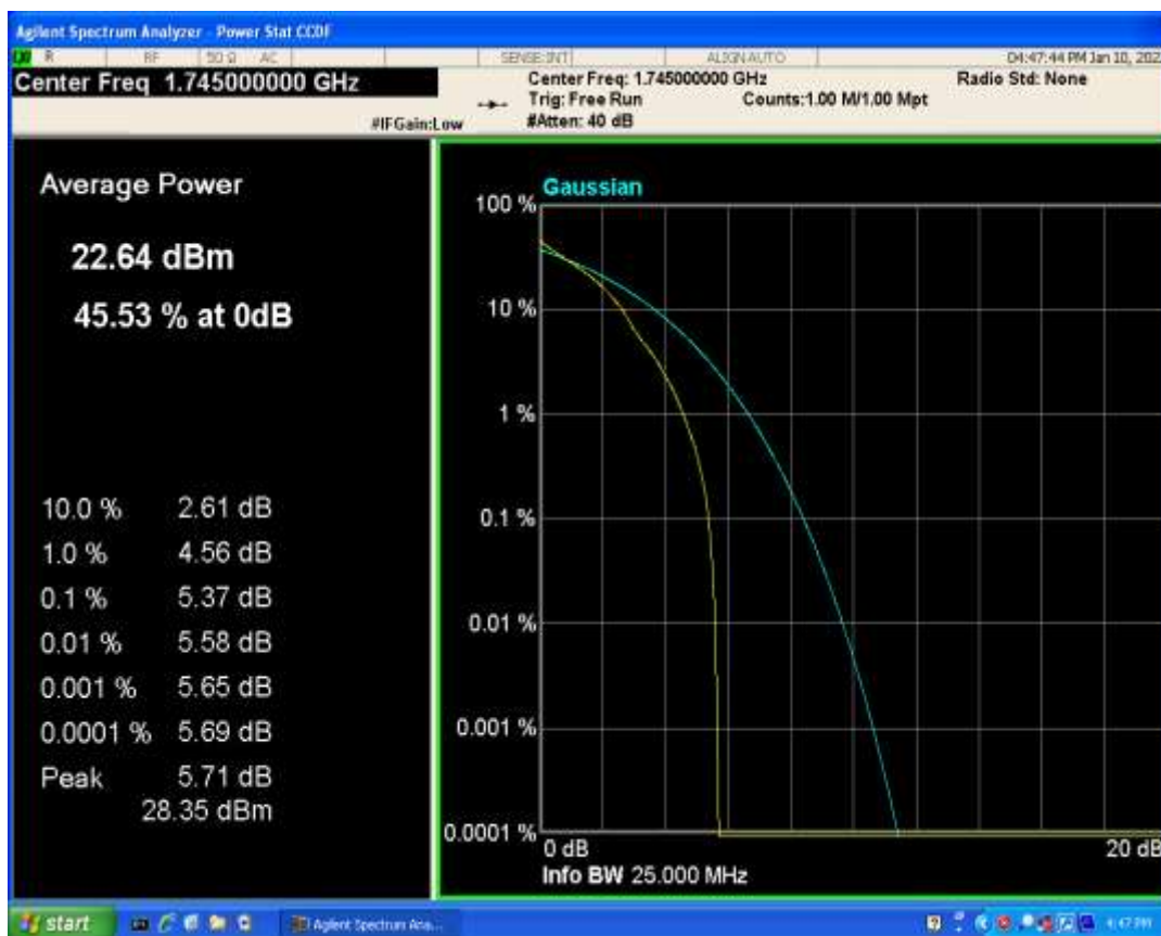
Band7 QAM16 BW=15MHz Channel=21100 RB Size=1 Position=#0
