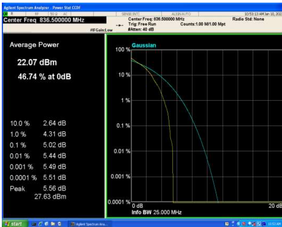
Band5 QAM16 BW=3MHz Channel=20525 RB Size=1 Position=#0
