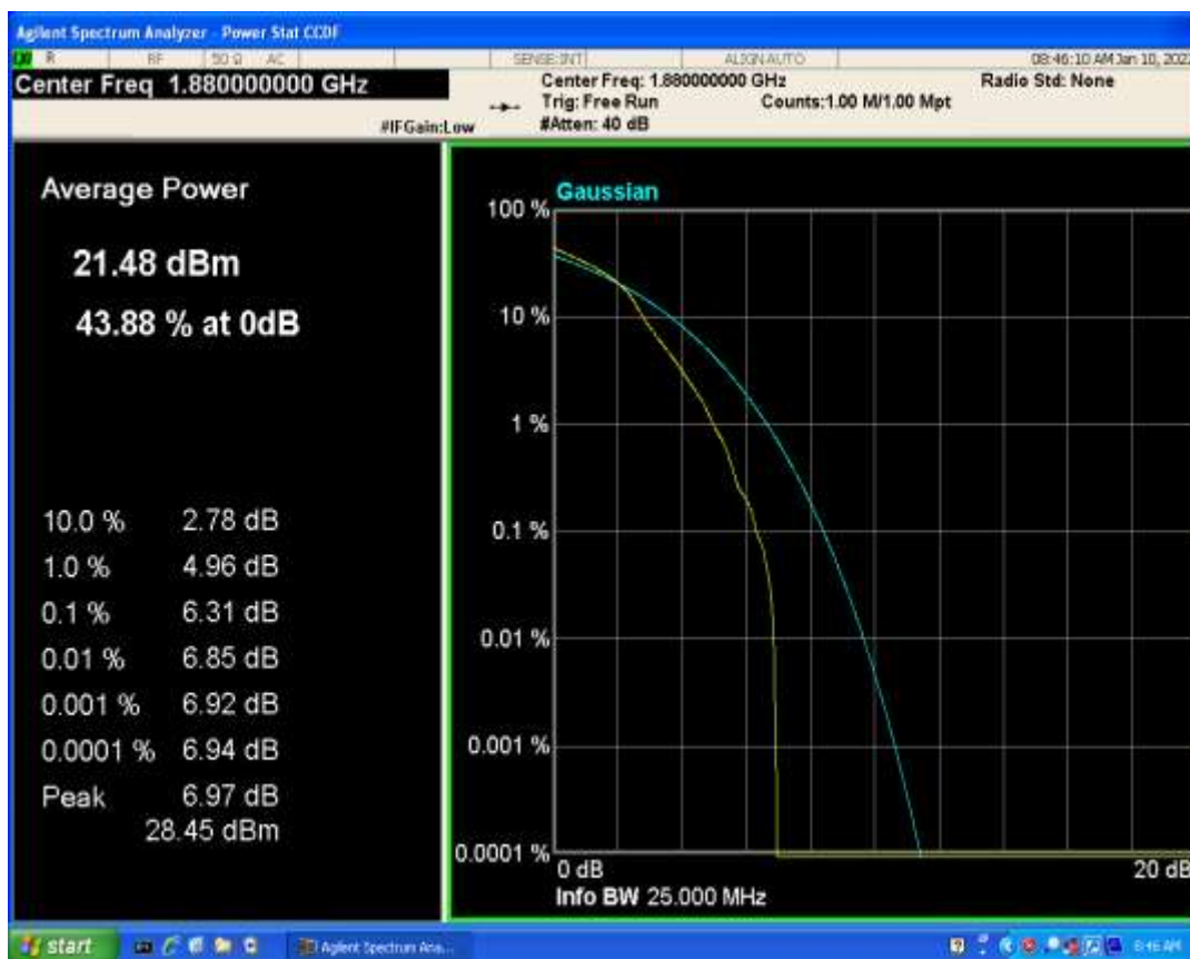
Band2 QPSK BW=15MHz Channel=18900 RB Size=1 Position=#0
