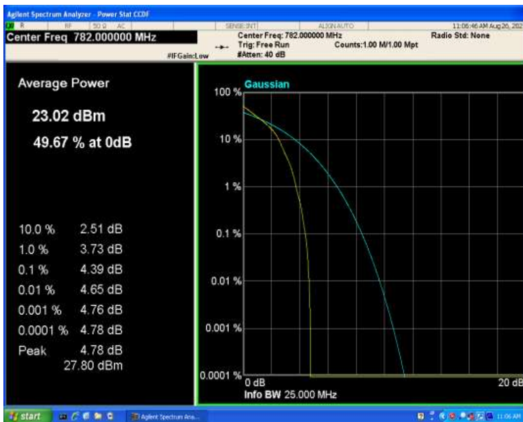
Band13 QAM16 BW=10MHz Channel=23230 RB Size=1 Position=#0
