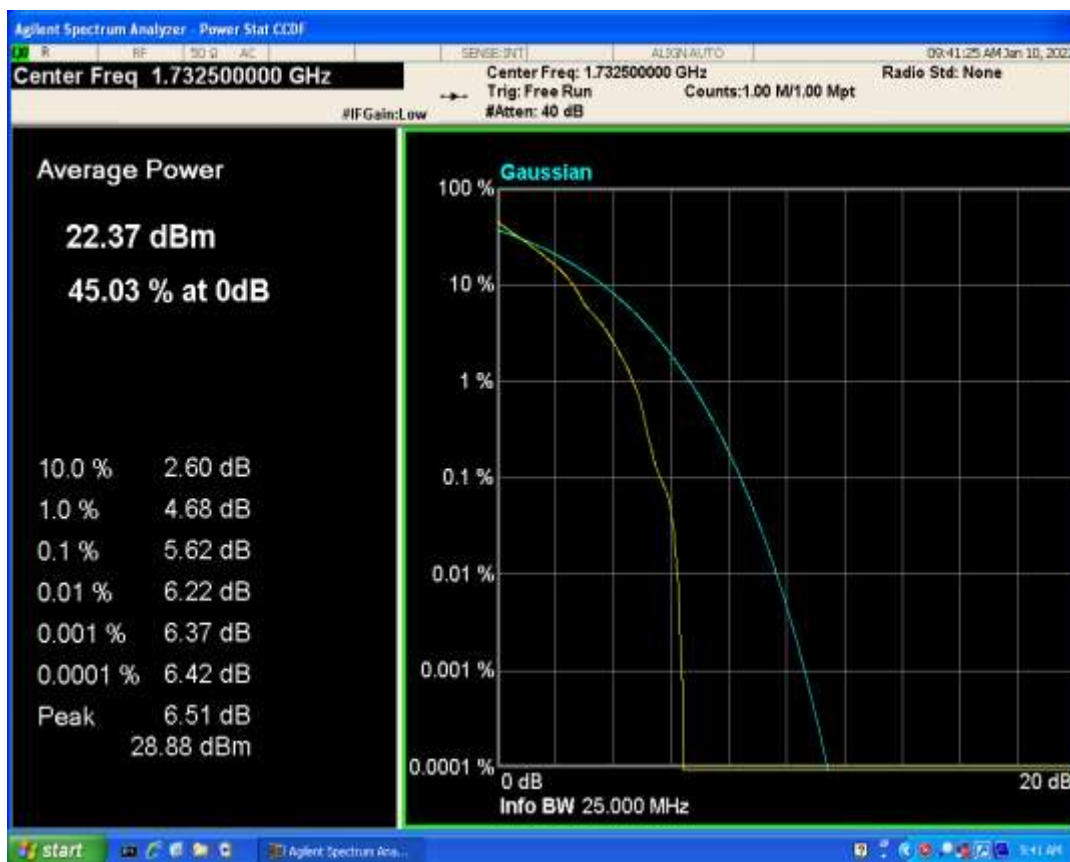
Band4 QPSK BW=3MHz Channel=20175 RB Size=1 Position=#0
