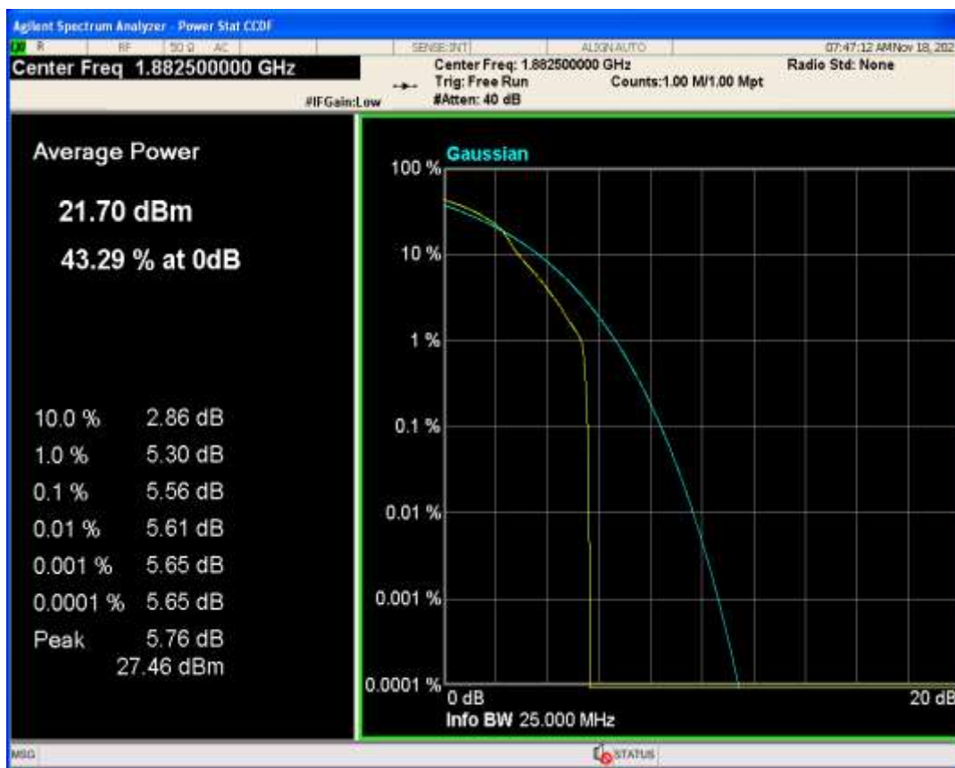
Band25 QPSK BW=20MHz Channel=26365 RB Size=1 Position=#0
