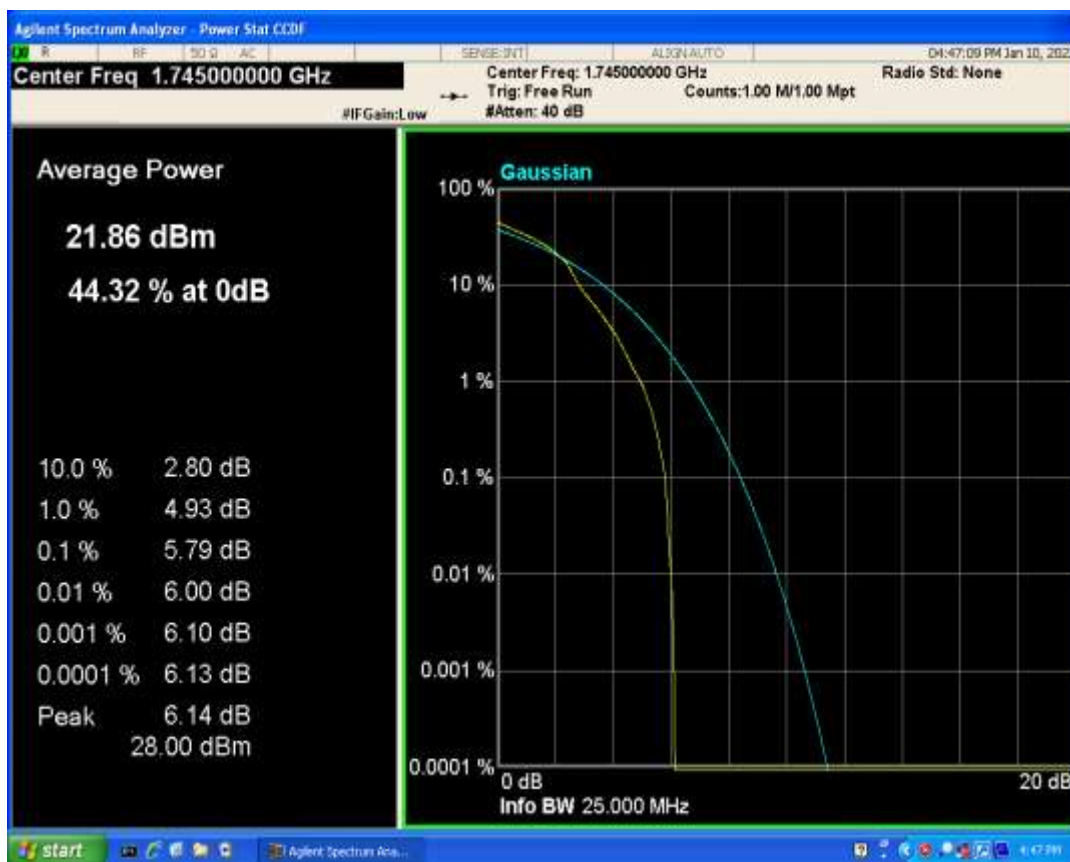
Band66 QPSK BW=5MHz Channel=132322 RB Size=1 Position=#0
