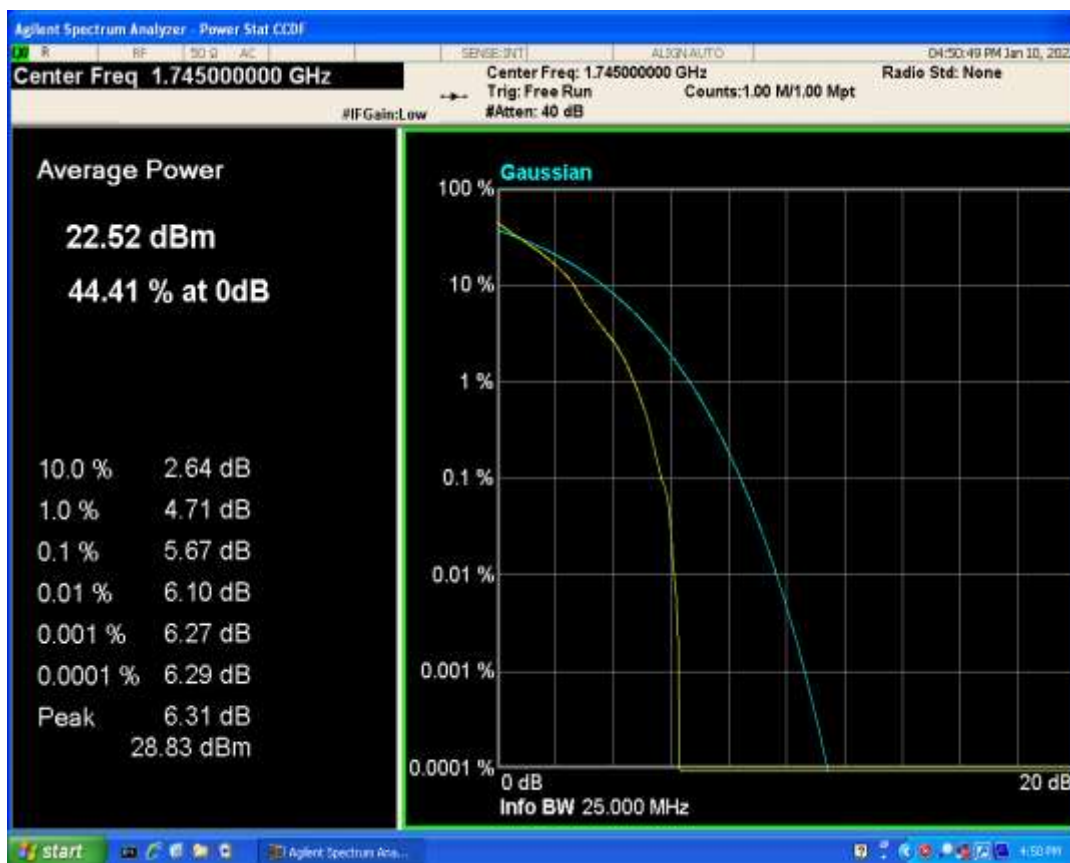
Band66 QPSK BW=1.4MHz Channel=132322 RB Size=1 Position=#0
