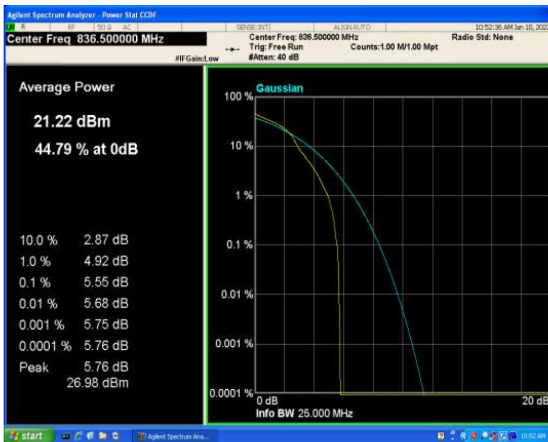
Band5 QAM16 BW=5MHz Channel=20525 RB Size=1 Position=#0
