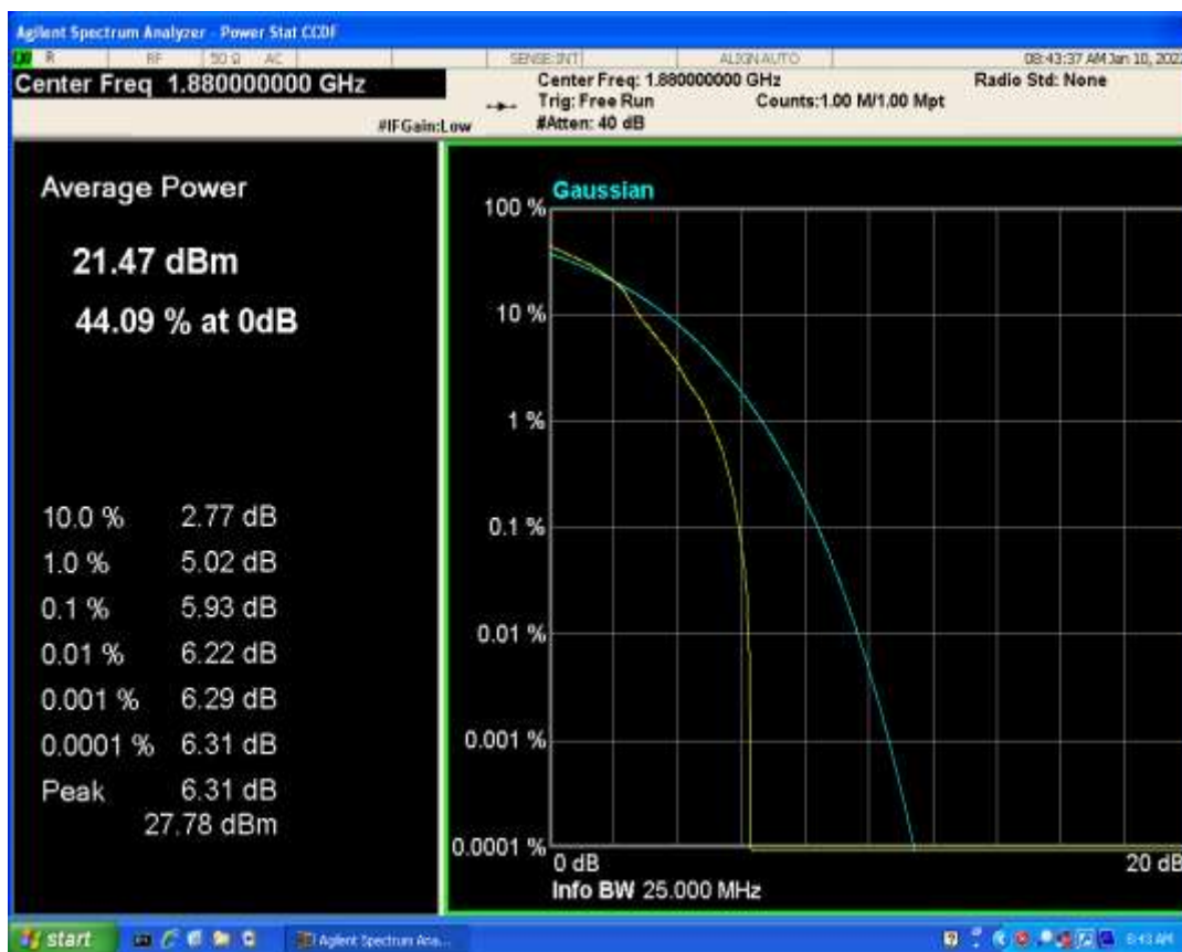
Band2 QAM16 BW=10MHz Channel=18900 RB Size=1 Position=#0
