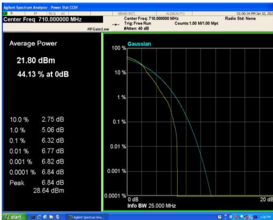
Band17 QPSK BW=5MHz Channel=23790 RB Size=1 Position=#0
