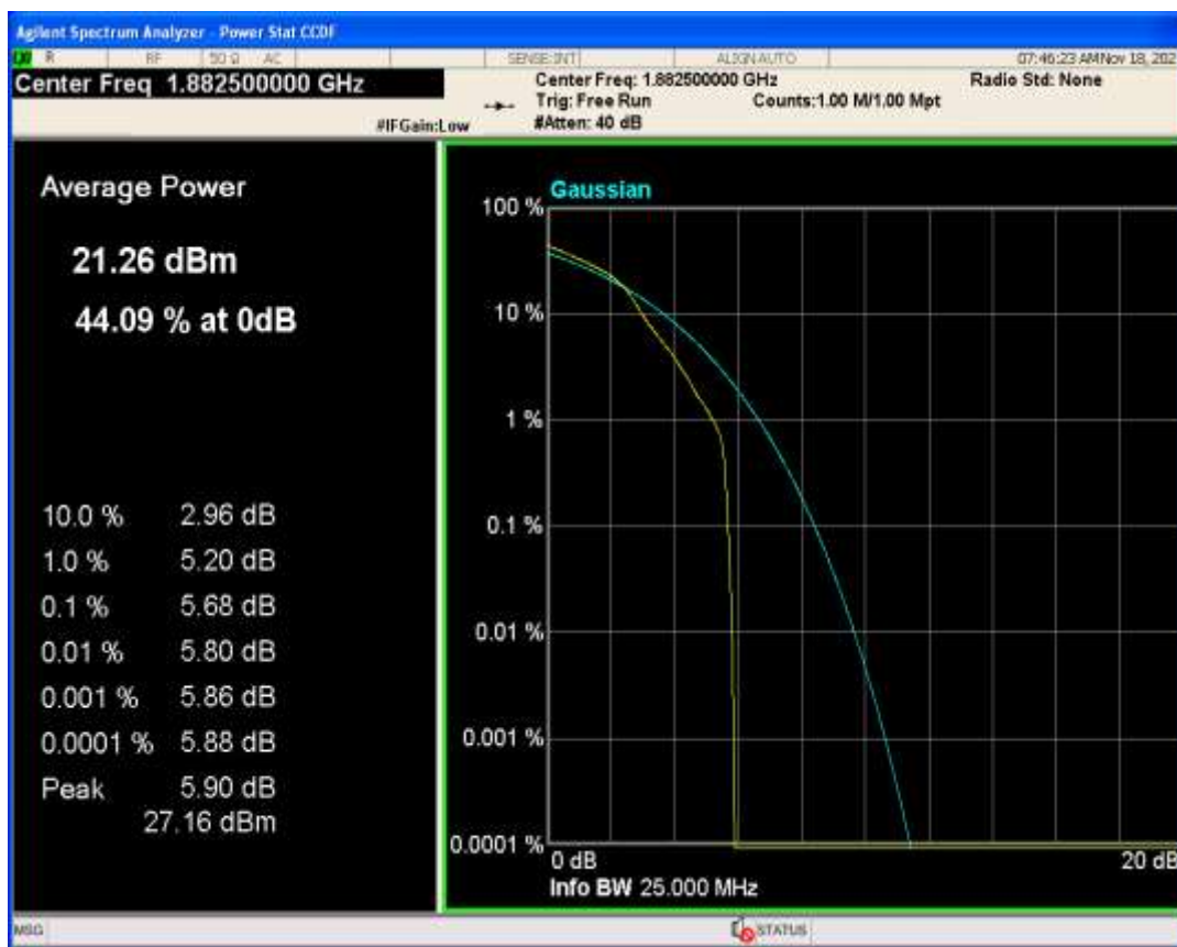
Band25 QAM16 BW=10MHz Channel=26365 RB Size=1 Position=#0
