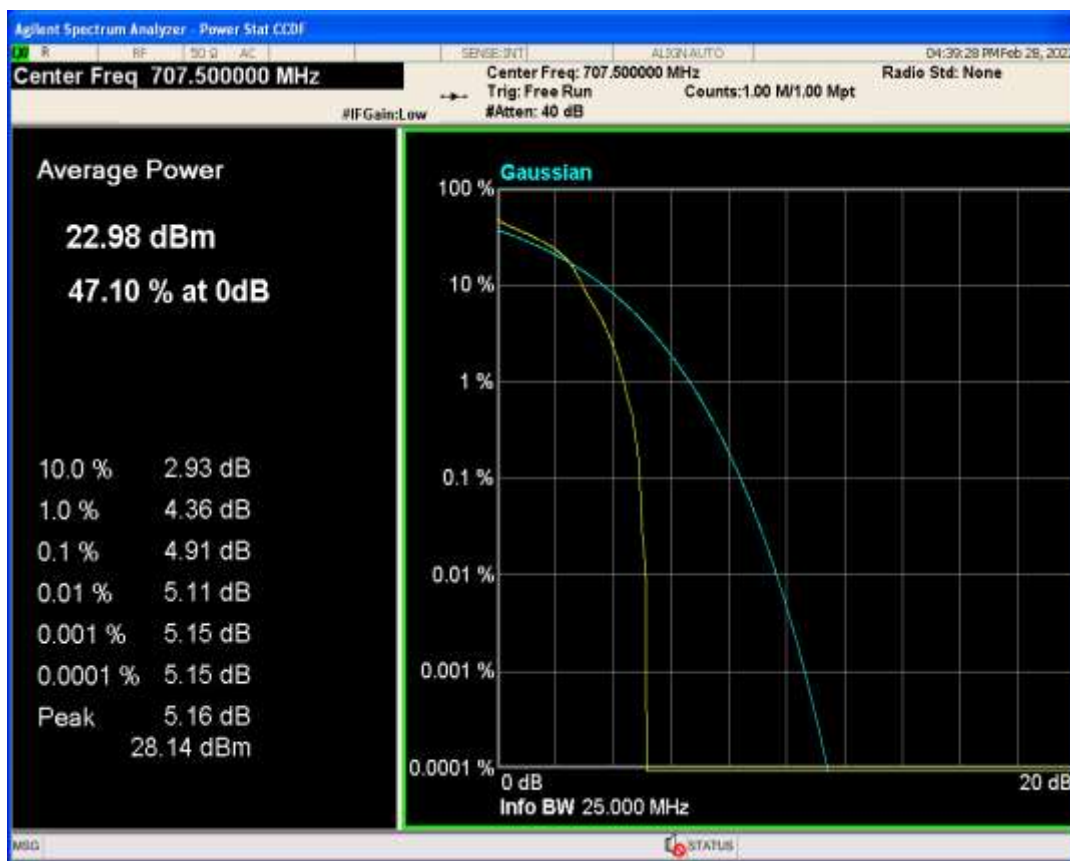
Band13 QPSK BW=10MHz Channel=23230 RB Size=1 Position=#0
