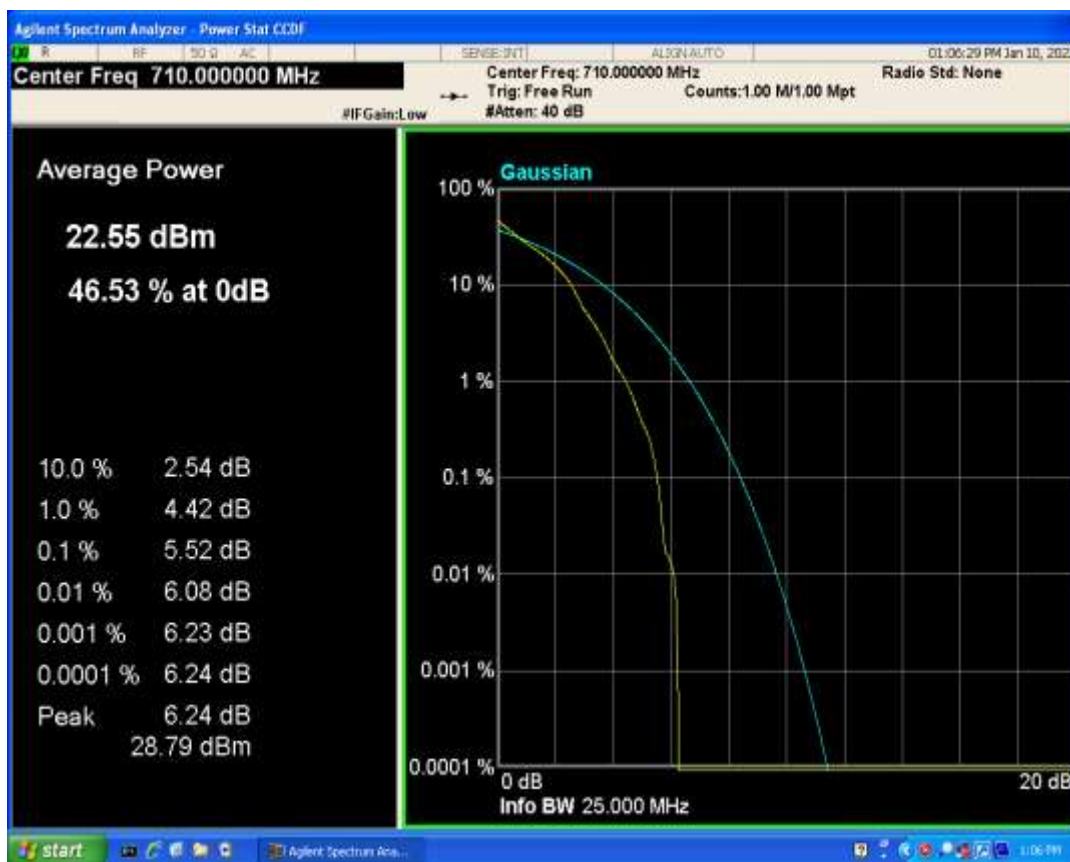
Band17 QAM16 BW=5MHz Channel=23790 RB Size=1 Position=#0
