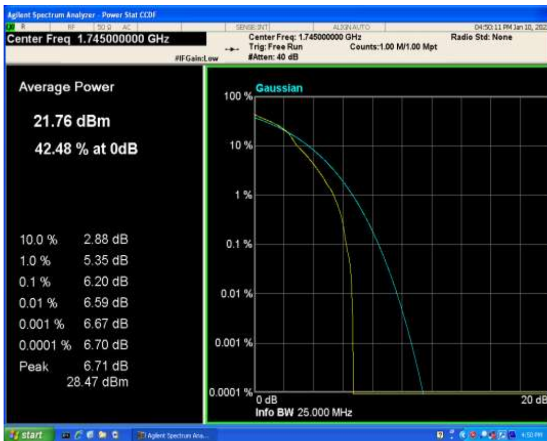
Band66 QAM16 BW=5MHz Channel=132322 RB Size=1 Position=#0
