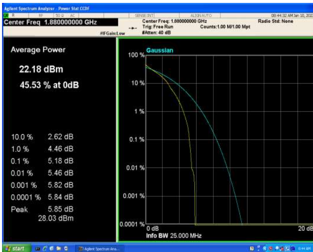
Band2 QPSK BW=3MHz Channel=18900 RB Size=1 Position=#0
