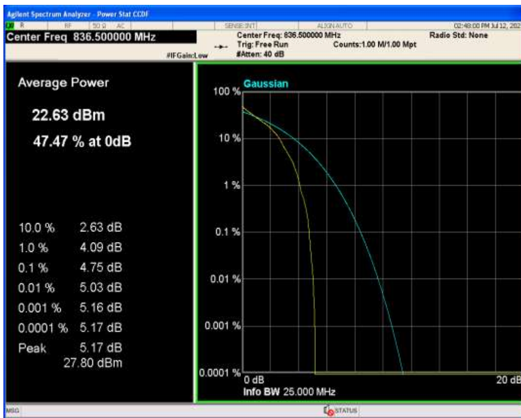
Band26b QAM16 BW=5MHz Channel=26915 RB Size=1 Position=#0
