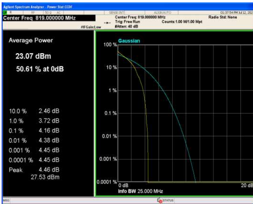
Band26a QAM16 BW=3MHz Channel=26740 RB Size=1 Position=#0
