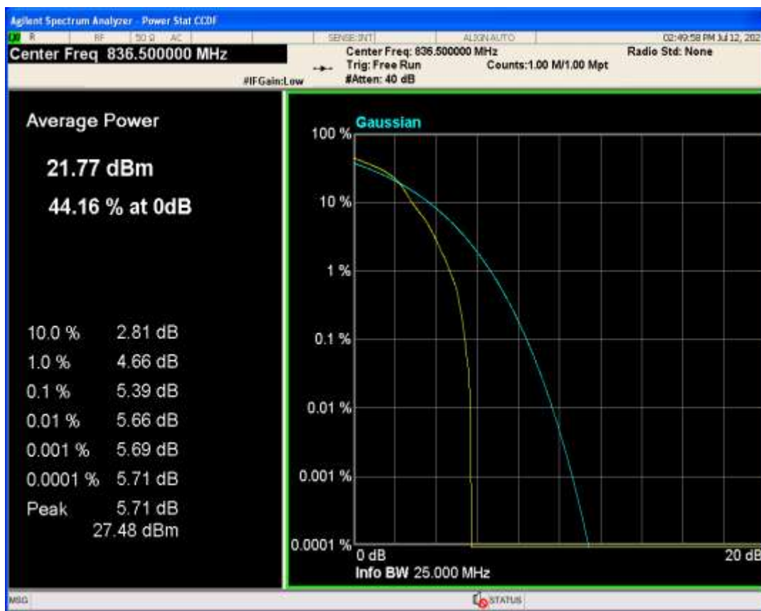
Band26b QAM16 BW=3MHz Channel=26915 RB Size=1 Position=#0
