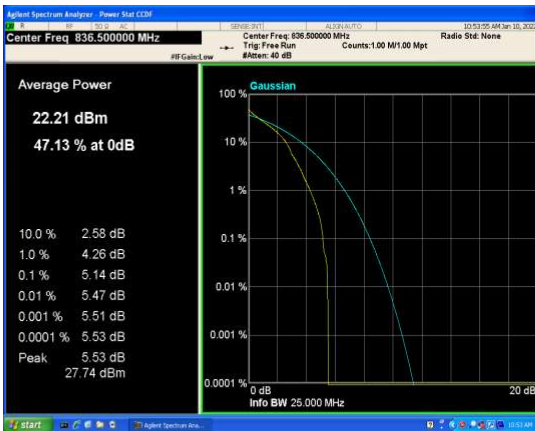
Band5 QPSK BW=3MHz Channel=20525 RB Size=1 Position=#0
