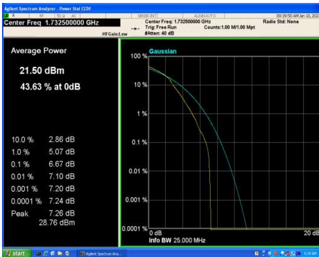
Band4 QAM16 BW=20MHz Channel=20175 RB Size=1 Position=#0
