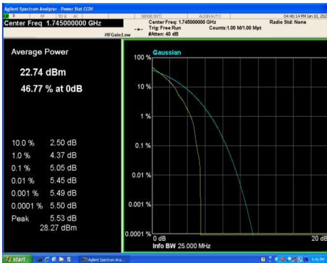
Band66 QAM16 BW=20MHz Channel=132322 RB Size=1 Position=#0
