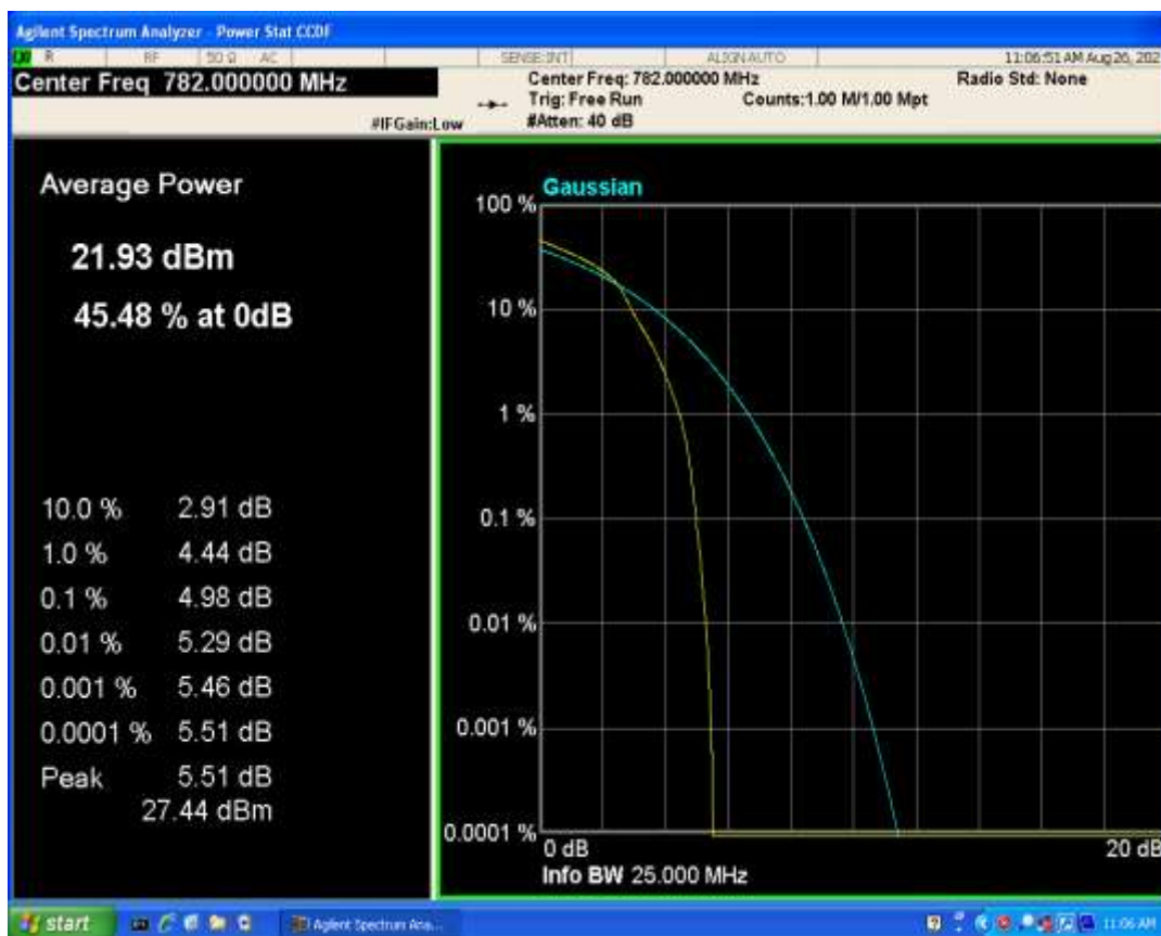
Band17 QAM16 BW=10MHz Channel=23790 RB Size=1 Position=#0
