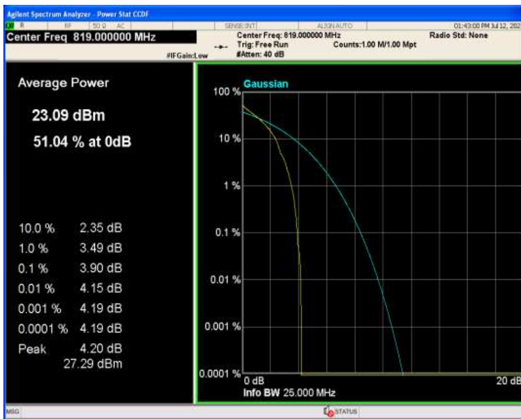
Band26b QAM16 BW=15MHz Channel=26915 RB Size=1 Position=#0
