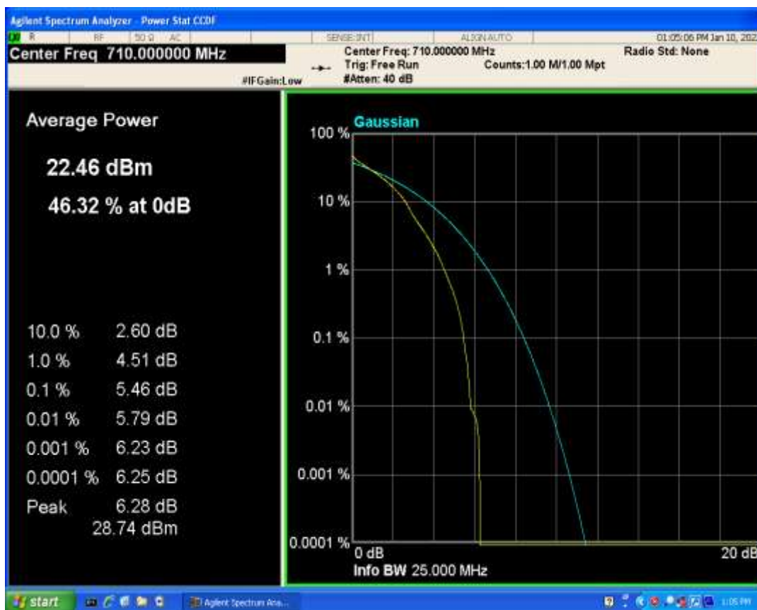
Band17 QPSK BW=10MHz Channel=23790 RB Size=1 Position=#0
