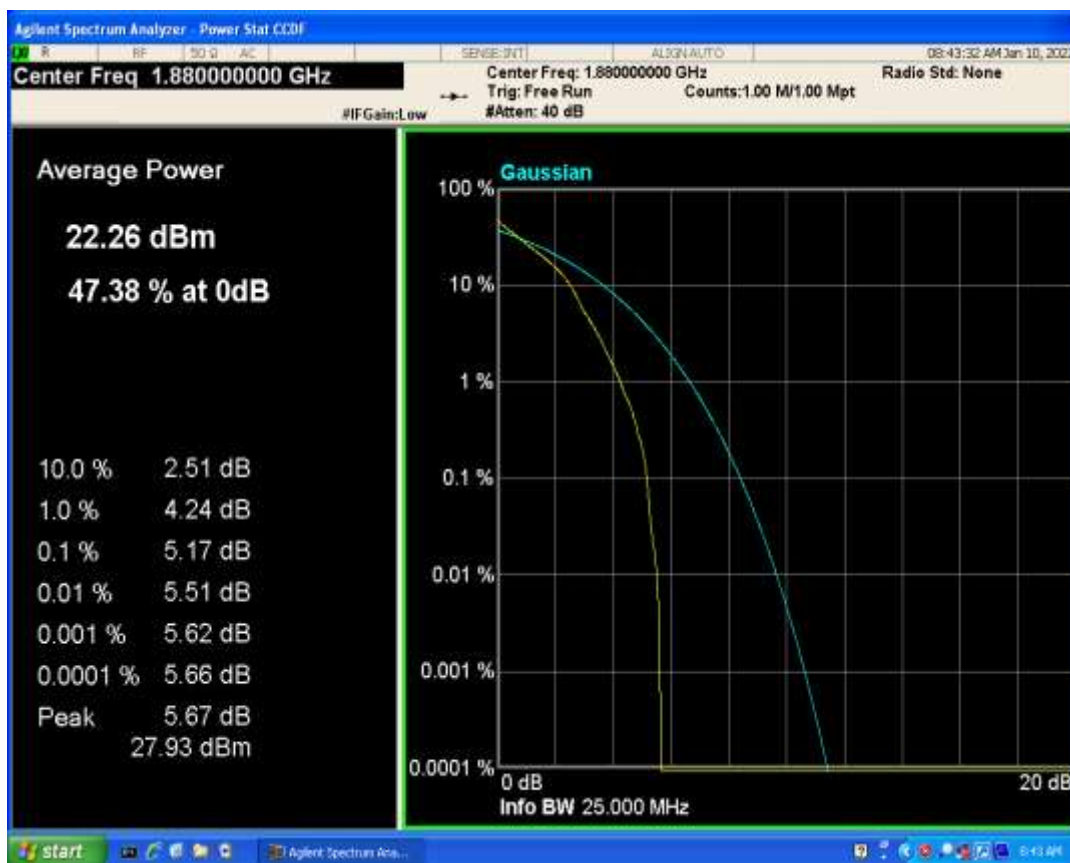
Band25 QAM16 BW=20MHz Channel=26365 RB Size=1 Position=#0
