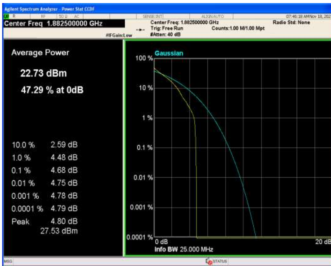
Band25 QPSK BW=10MHz Channel=26365 RB Size=1 Position=#0
