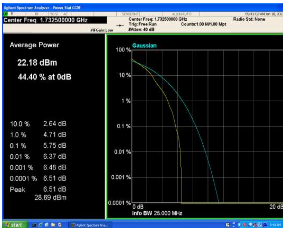
Band4 QAM16 BW=3MHz Channel=20175 RB Size=1 Position=#0
