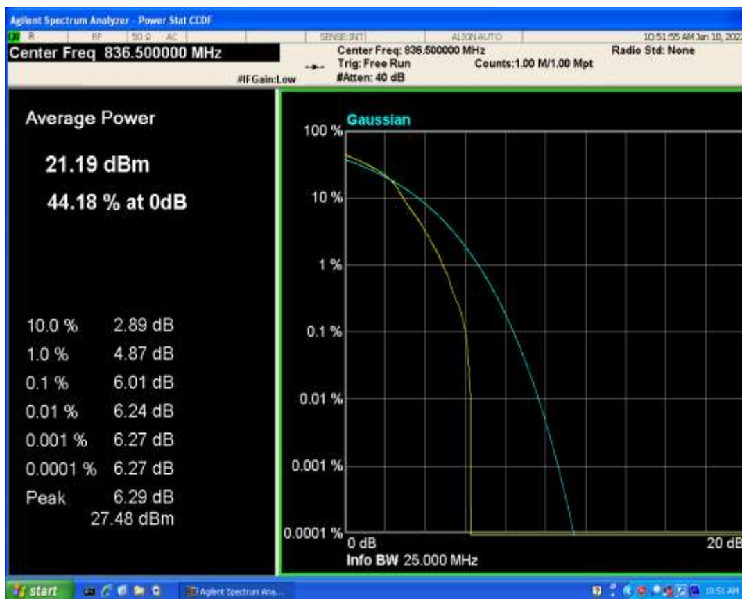
Band5 QPSK BW=10MHz Channel=20525 RB Size=1 Position=#0
