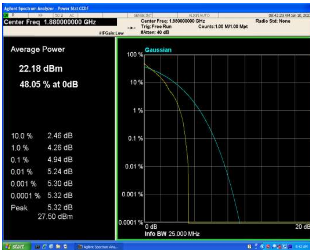
Band2 QPSK BW=5MHz Channel=18900 RB Size=1 Position=#0
