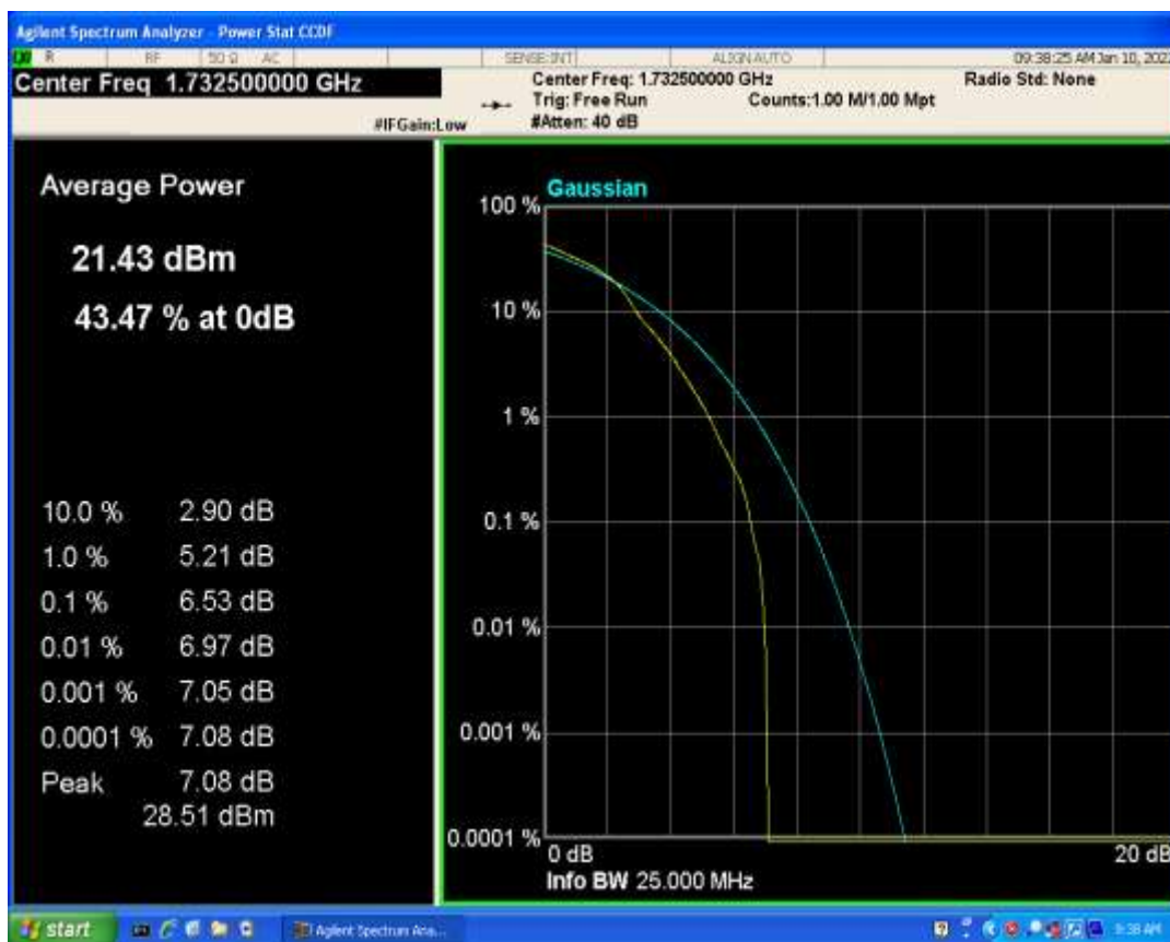
Band4 QPSK BW=15MHz Channel=20175 RB Size=1 Position=#0
