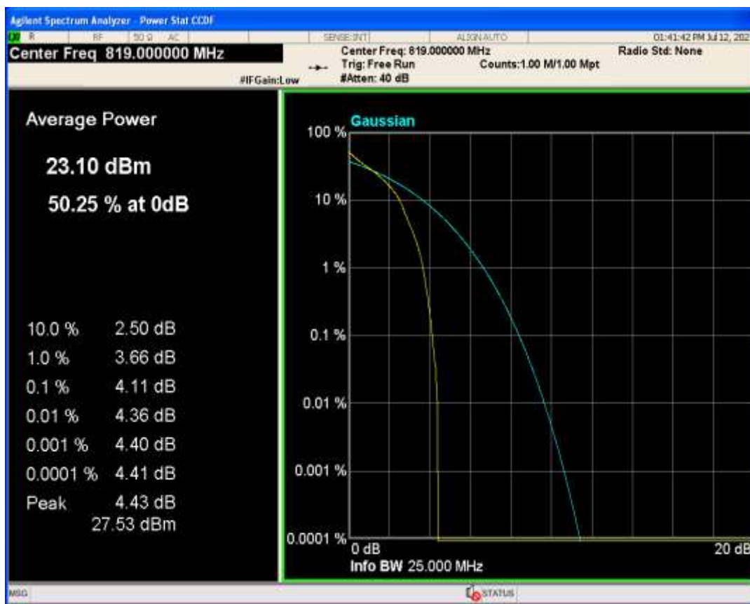
Band26a QPSK BW=3MHz Channel=26740 RB Size=1 Position=#0
