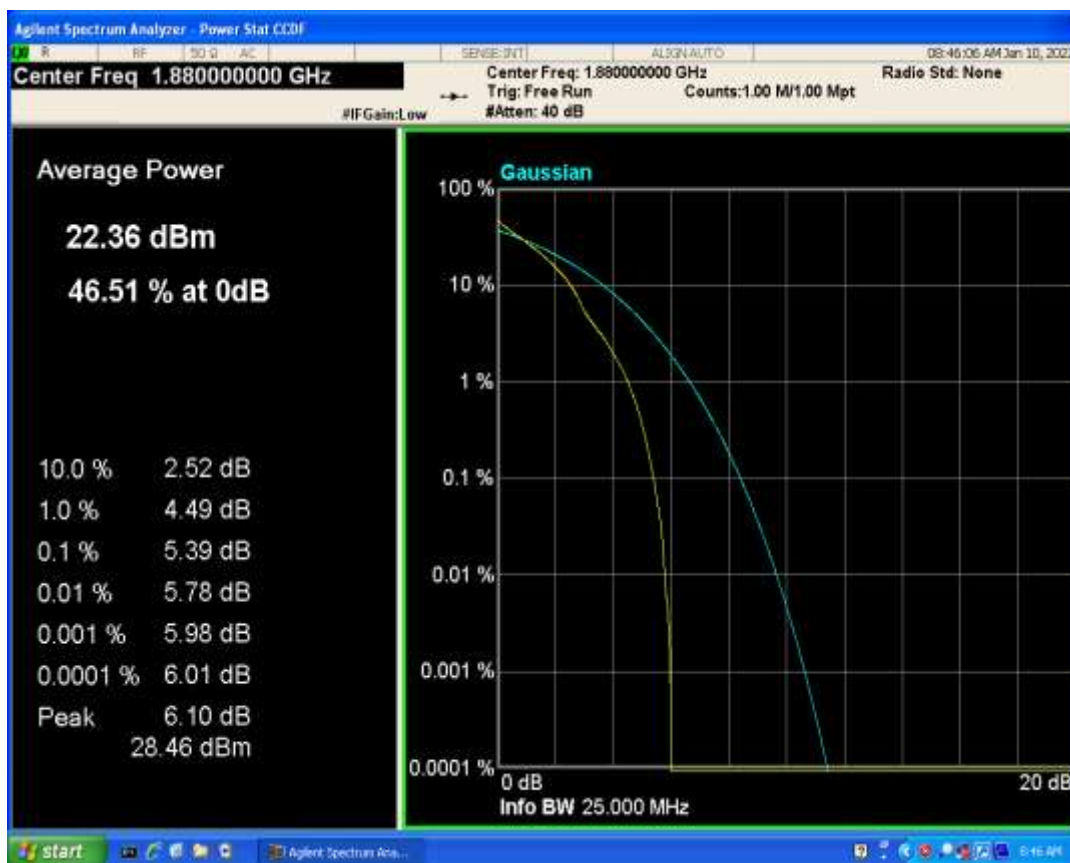
Band2 QPSK BW=20MHz Channel=18900 RB Size=1 Position=#0
