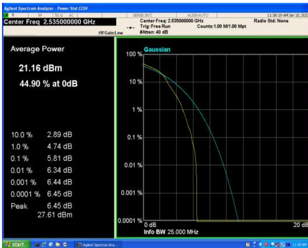
Band7 QAM16 BW=10MHz Channel=21100 RB Size=1 Position=#0
