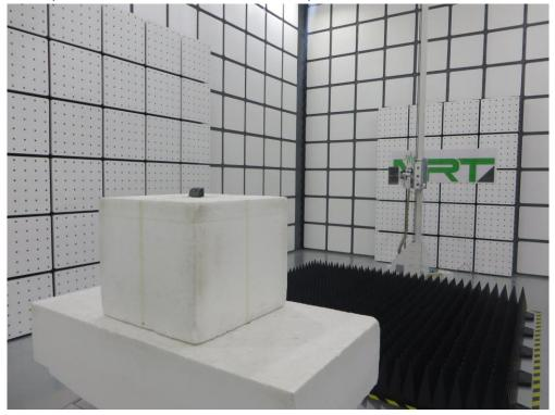
Note: The edge of test table align with the center of turn table.
