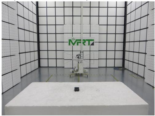
Description: Radiated Emissions Test Setup for 1~18GHz
