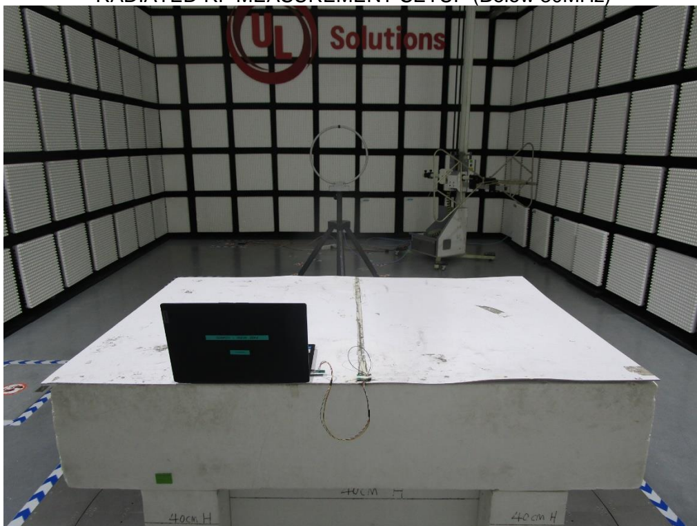
RADIATED RF MEASUREMENT SETUP (Below 30MHz)
