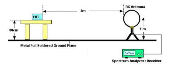
(B) Radiated Emission Test-Up Frequency 30MHz~1GHz
