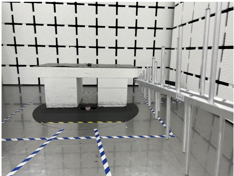
Radiation Emission Test Setup (30MHz to 1GHz)
