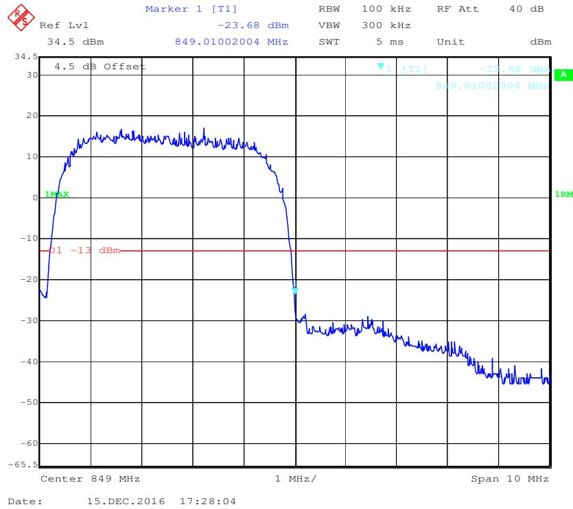
**Cellular Band, Left Band Edge for HSDPA (16QAM) Mode**
