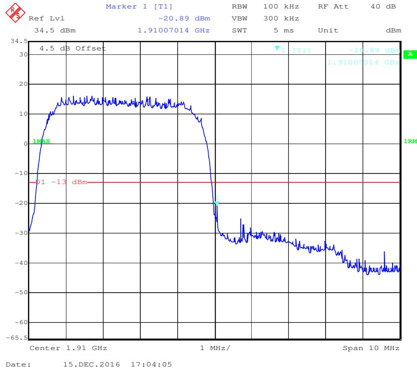
**PCS Band, Left Band Edge for HSDPA (16QAM) Mode**
