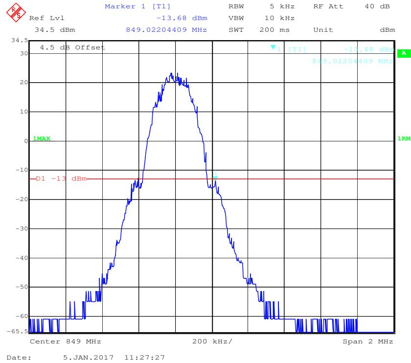
**Cellular Band, Left Band Edge for WCDMA (BPSK) Mode**
