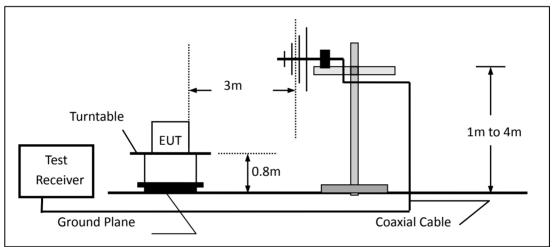
(c) For radiated emissions above 1000MHz
