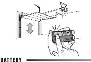
The LED(s) on your remote control will stop flashing when the battery is low and needs to be replaced. To replace battery, open the case as shown. Insert battery positive side up (+). Replace the battery with only 3V2032 or 3V2016 coin cell batteries (depending on the model). Dispose of old battery properly.
