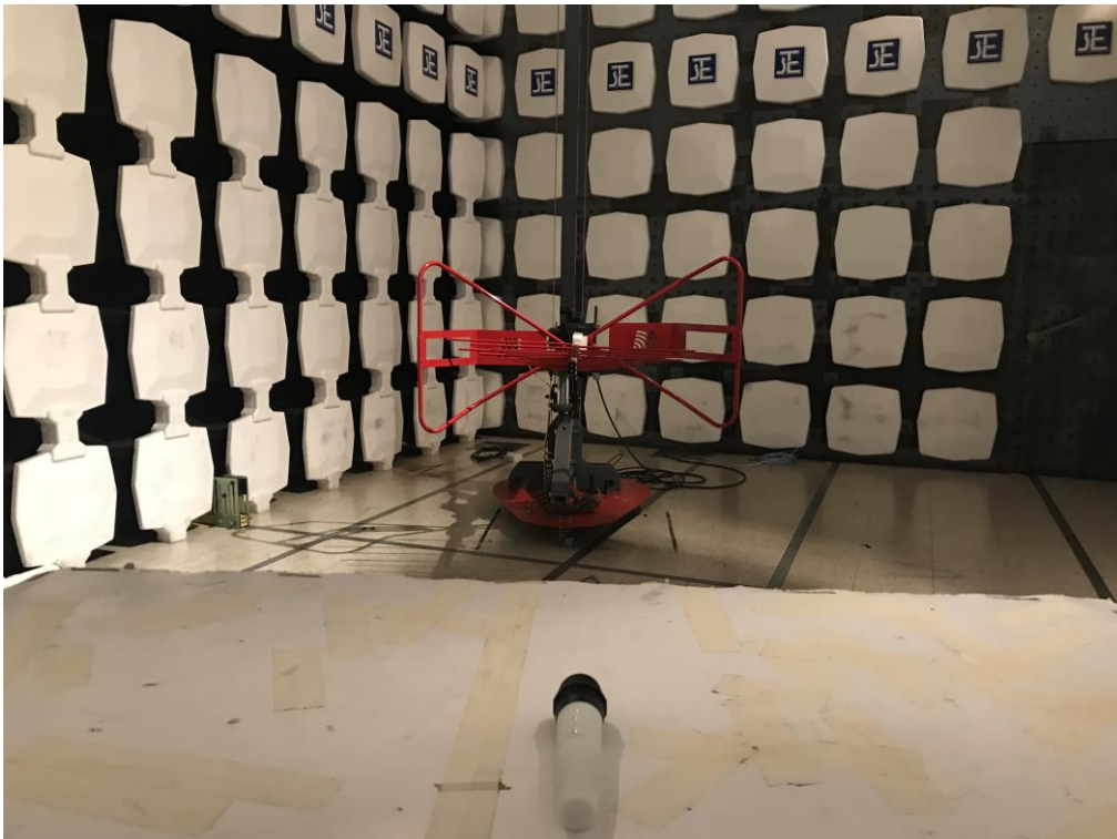
Measurement of Radiated Emission Test Set Up
