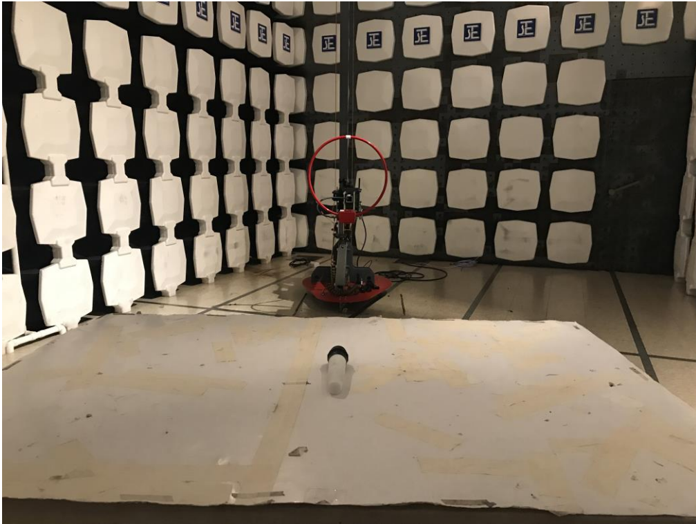
Measurement of Radiated Emission Test Set Up
