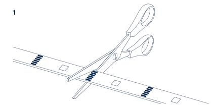
The length of Light Strip Pro can be adjusted to accommodate your chosen application (maximum strip length 2000 mm | 78.8 in). To shorten Light Strip Pro, use a pair of scissors to bisect the oval copper pads.
