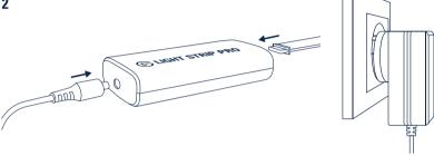
Connect the LED strip to the controller. Then connect the controller to the power supply and plug it into a power outlet.
