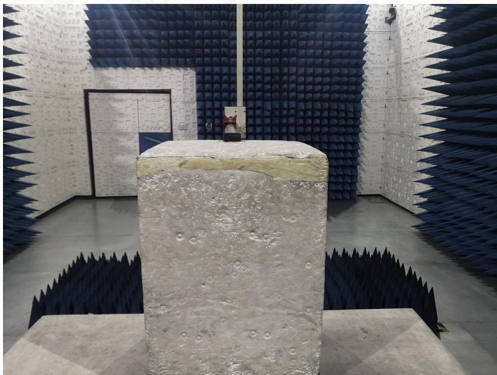
FCC RADIATED EMISSION TEST SETUP ABOVE 1GHZ
