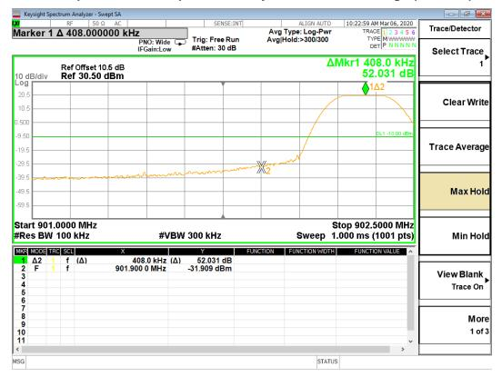
Screen Capture from the spectrum analyzer: Upper Band Edge (125 KHz)
