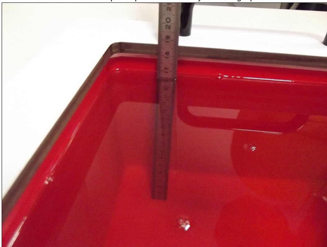
Photo 1: Liquid depth 450 MHz body simulating liquid
