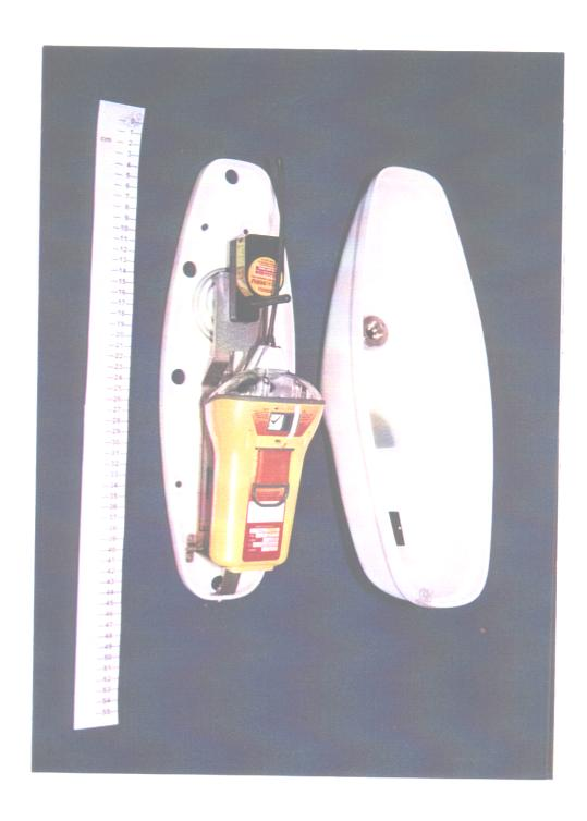
Float Free Enclosure with cover removed (Pains-Wessex HRU installed)
