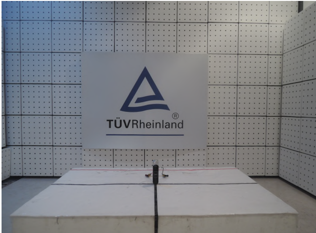
Photograph 2: Set-up for Radiated Emissions (Back View 1)
