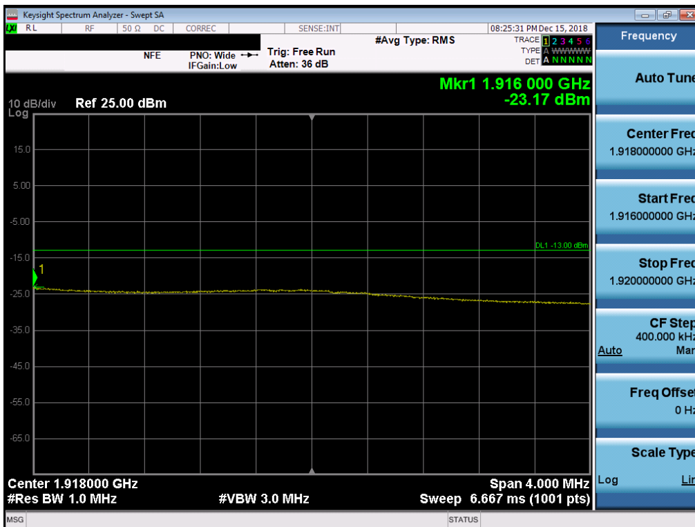
Plot 7-146. Upper Extended Band Edge Plot (Band 25 - 15.0MHz QPSK - Full RB Configuration)
