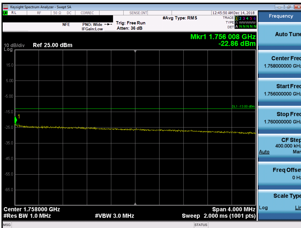
Plot 7-108. Upper Extended Band Edge Plot (Band 4 - 10.0MHz QPSK - Full RB Configuration)
