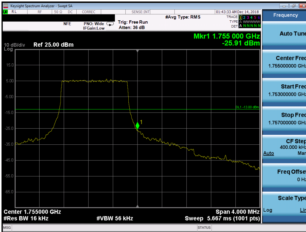
Plot 7-95. Upper Band Edge Plot (Band 4 - 1.4MHz QPSK - Full RB Configuration)
