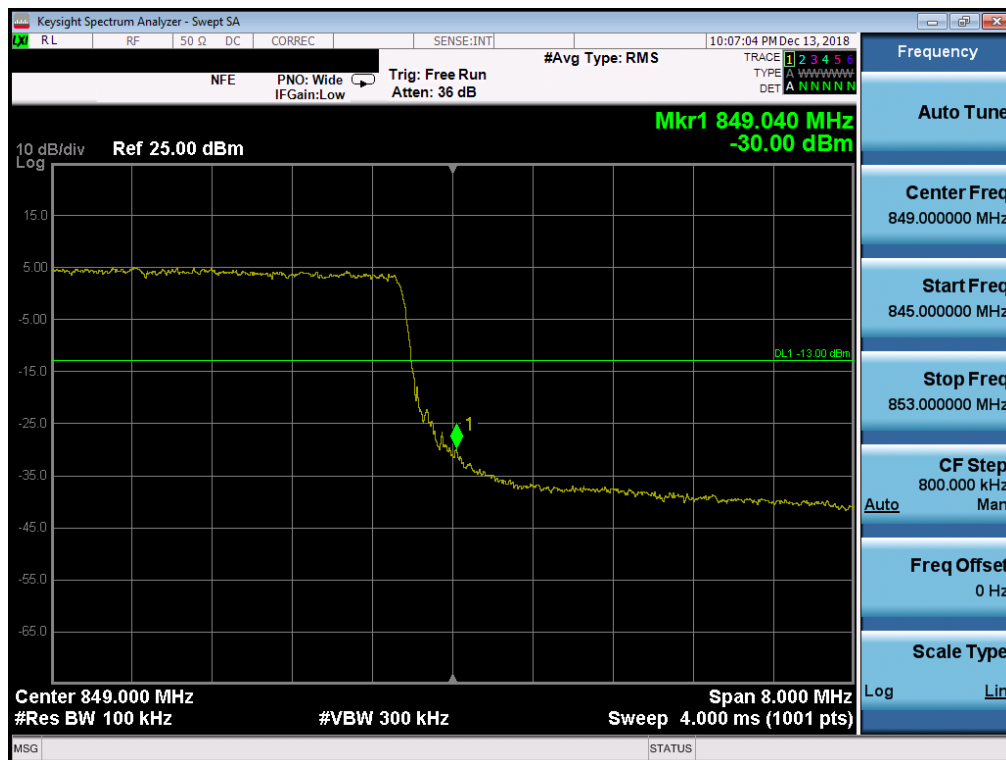
Plot 7-92. Upper Band Edge Plot (Band 5 - 10.0MHz QPSK - Full RB Configuration)
