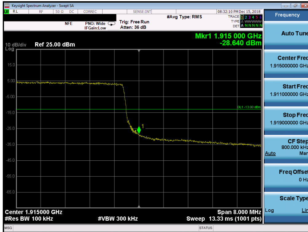
Plot 7-139. Upper Band Edge Plot (Band 25 - 10.0MHz QPSK - Full RB Configuration)
