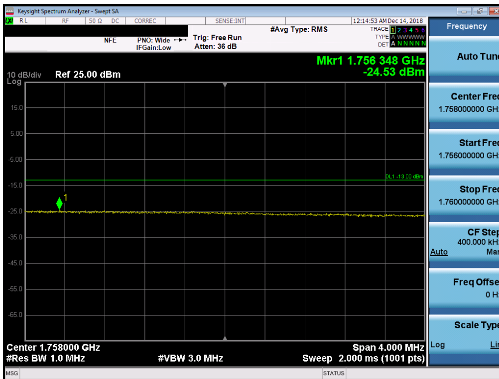
Plot 7-116. Upper Extended Band Edge Plot (Band 4 - 20.0MHz QPSK - Full RB Configuration)
