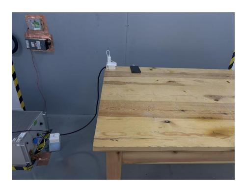
Set-up for Radiated Emission (RE), Below 1GHz
