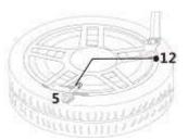
2.4 Final inspection: Visually inspect the rim, valve stem and electronic module to ensure no damage has occurred.
