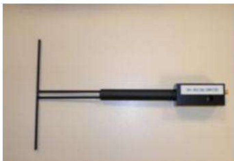
Figure 1 – Satimo COMOSAR Validation Dipole
