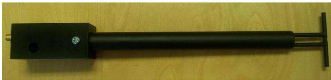
Figure 1 – MVG COMOSAR Validation Dipole
