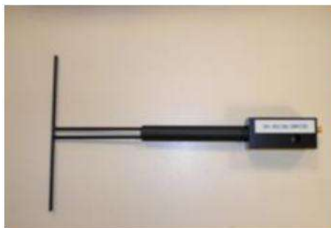
Figure 1 – Satimo COMOSAR Validation Dipole
