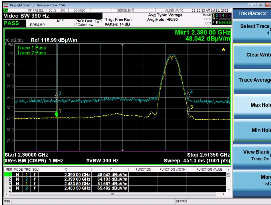
**Graph 5: Radiated Higher Band Edge Plot b-Mode – 2472 MHz**
