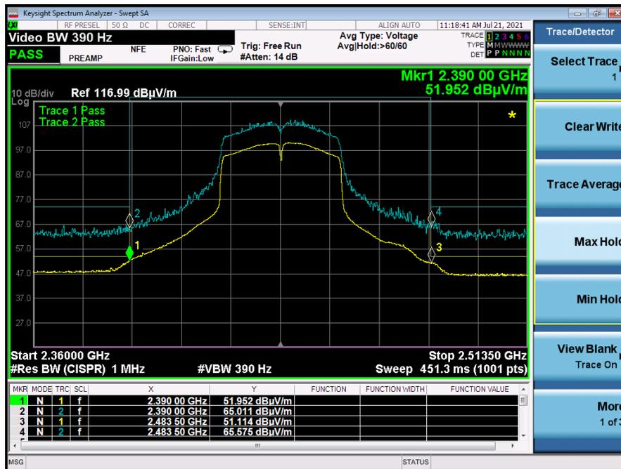
Graph 13: Radiated Middle Band Edge Plot n40-Mode – 2437 MHz
