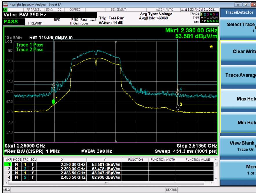
Graph 12: Radiated Lower Band Edge Plot n40-Mode – 2422 MHz
