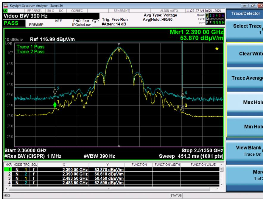
**Graph 4: Radiated Middle Band Edge Plot b-Mode – 2437 MHz**
