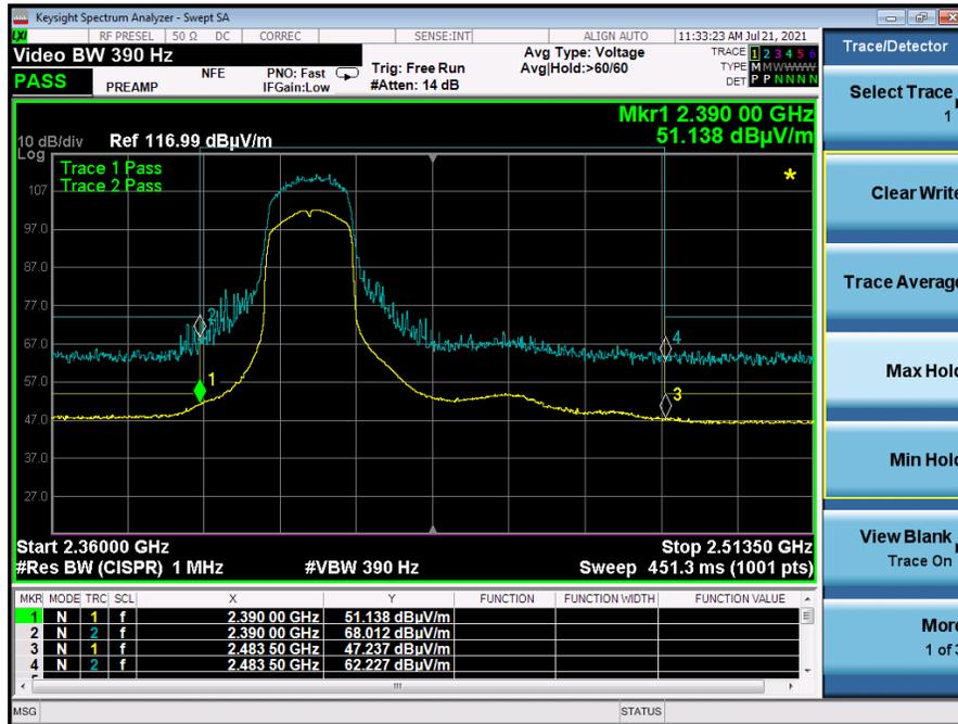
Graph 6: Radiated Lower Band Edge Plot g-Mode – 2412 MHz
