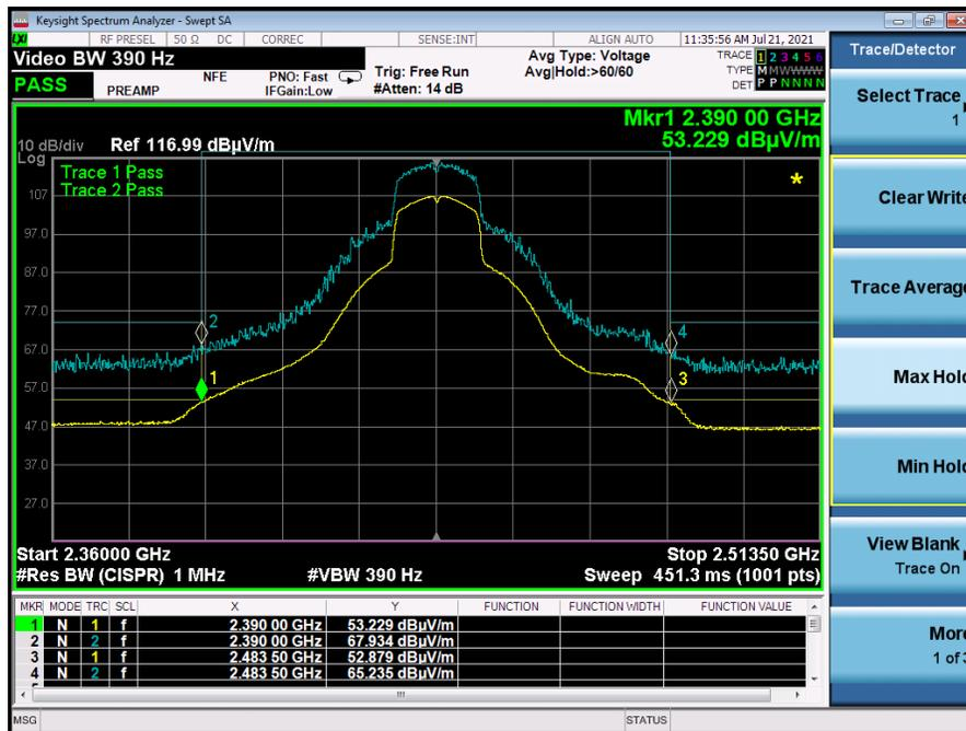
Graph 7: Radiated Middle Band Edge Plot g-Mode – 2437 MHz
