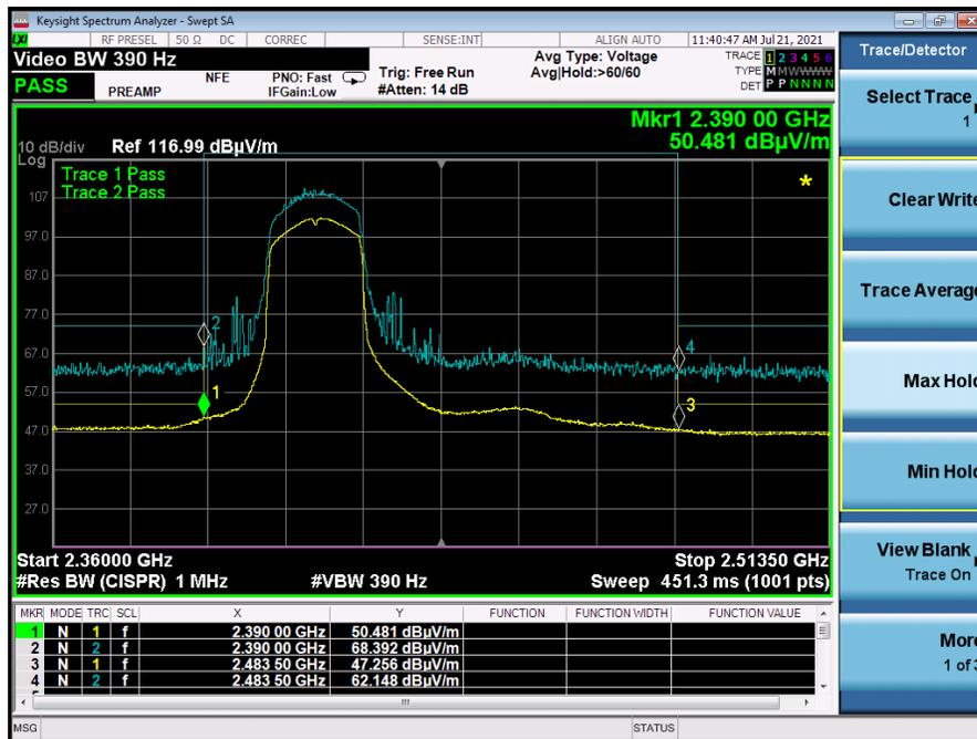
Graph 9: Radiated Lower Band Edge Plot n20-Mode – 2412 MHz
