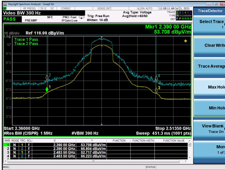
Graph 10: Radiated Middle Band Edge Plot n20-Mode – 2437 MHz
