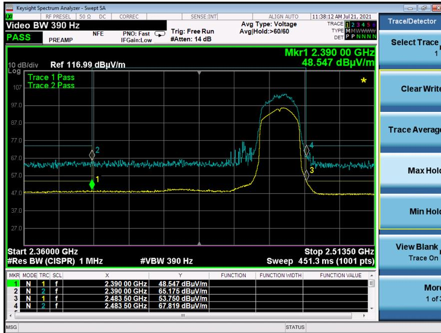
Graph 8: Radiated Higher Band Edge Plot g-Mode – 2472 MHz
