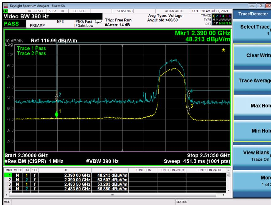
Graph 11: Radiated Higher Band Edge Plot n20-Mode – 2472 MHz
