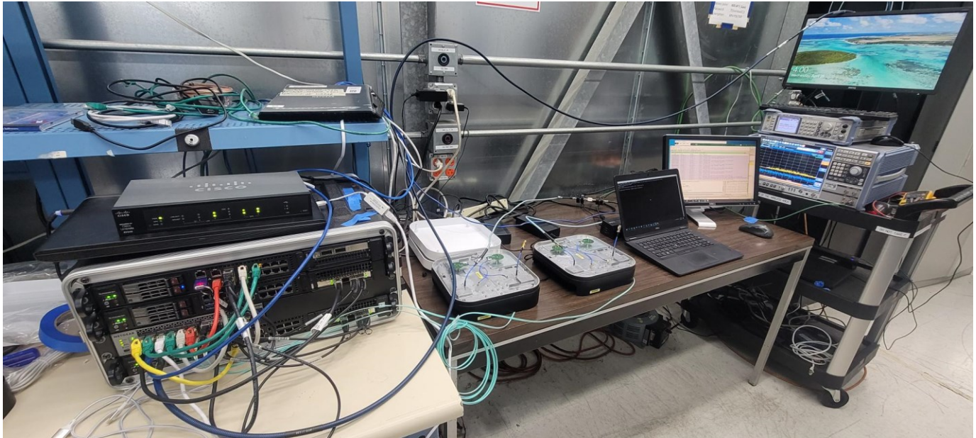
Figure 1 –Test setup – conducted antenna port tests
