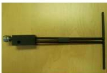
Figure 1 – MVG COMOSAR Validation Dipole
