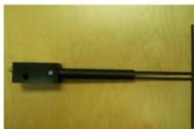
Figure 1 – MVG COMOSAR Validation Dipole
