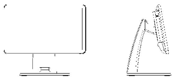
Single screen, length×width×height: 380mm\*198mm\*327mm; main screen flip angle 0-45°
