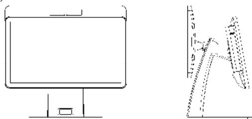
15.6-inch main screen + 15.6-inch secondary screen, length × width × height: 380mm\*205mm\*362mm; main screen flip angle 0-45°, secondary screen flip angle 0-30°
