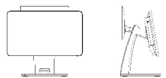
15.6-inch main screen + 10.1-inch secondary screen, length×width×height: 380mm\*205mm\*353mm; the flip angle of the main screen is 0-45°, and the flip angle of the secondary screen is 0-30°
