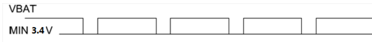
Figure 11 VBAT lowest voltage drop
