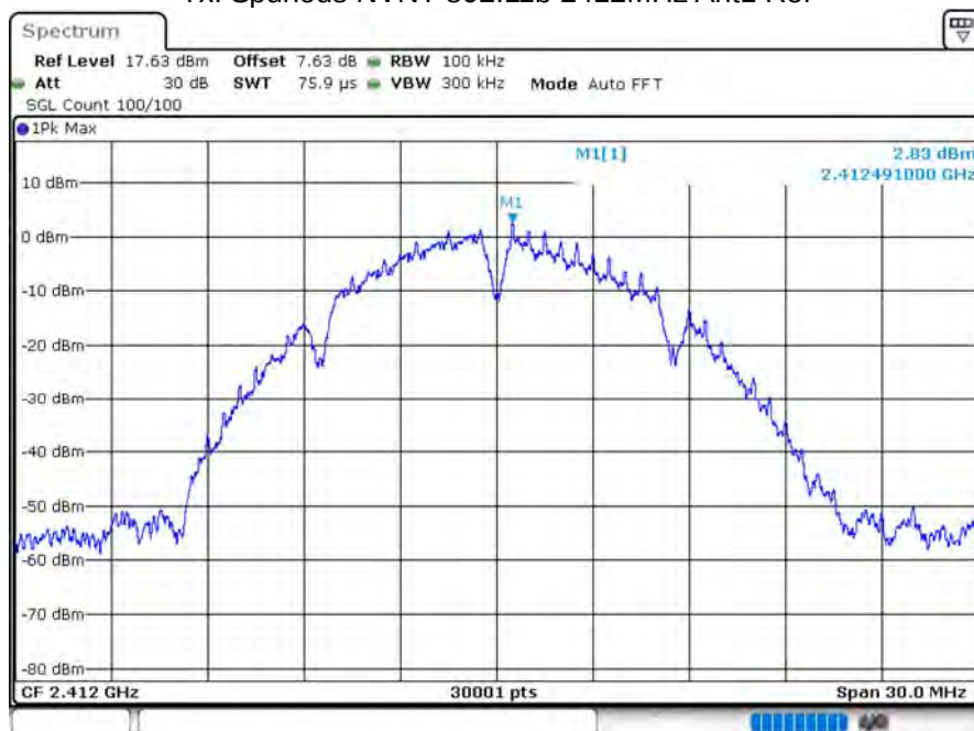
Tx. Spurious NVNT 802.11b 2412MHz Ant1 Ref
