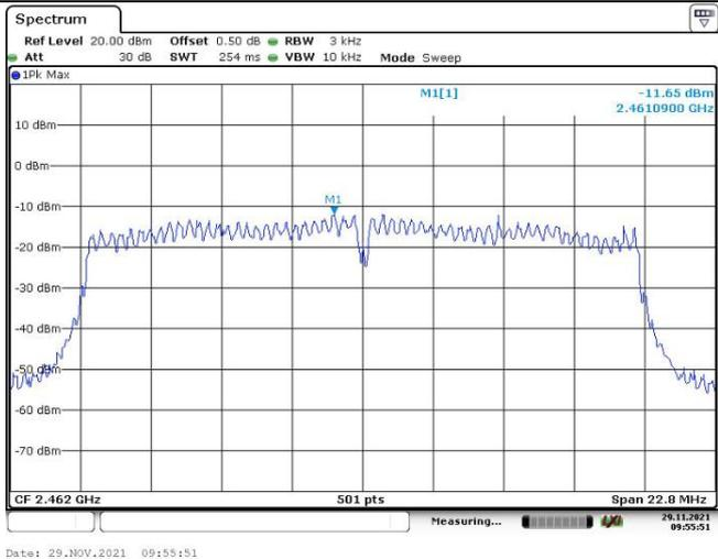
**4.7 100 kHz Bandwidth of Frequency Band Edge:**
