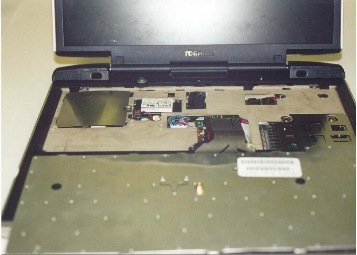
View of the WLAN Transmitter Location Inside the Tecra Laptop
