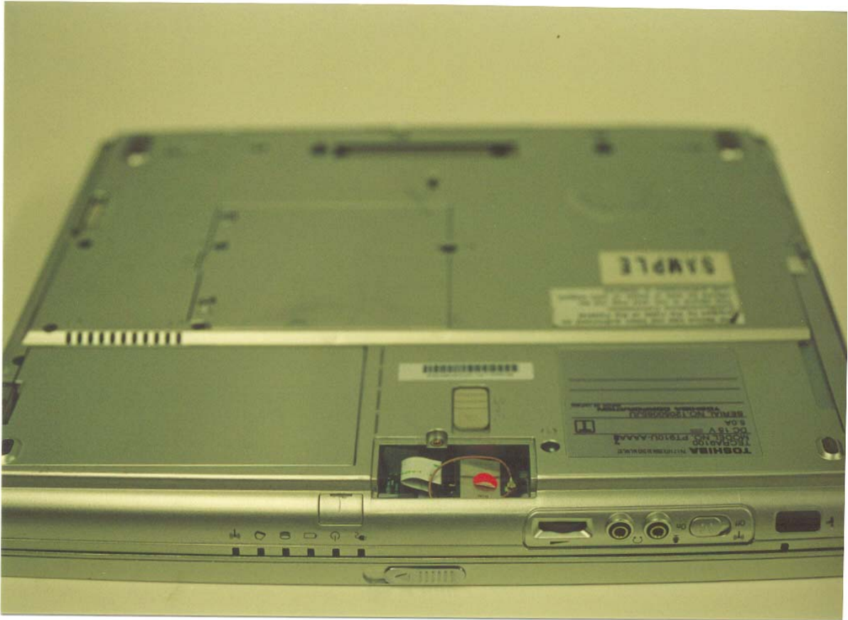
View of Bluetooth Transmitter Location Inside the Tecra Laptop
